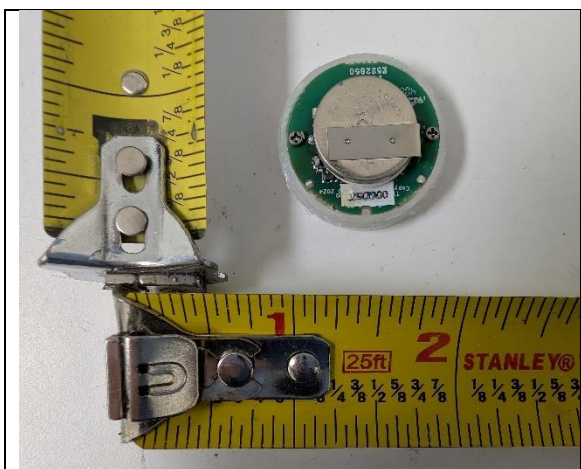
EUT Tot Tag, - (periodic transmission) -Internal View with Battery
