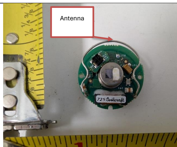
EUT Tot Tag, - (periodic transmission) -Internal View (Front)
