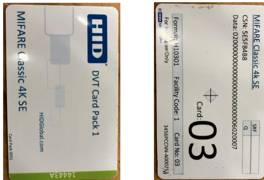
Figure 2: Front / Back Photo of the 13.56MHz RFID Credential
