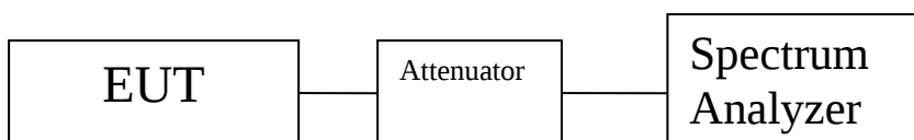
Figure 18: Block Diagram, Occupied Bandwidth Test Setup
