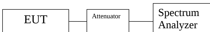
Figure 156: Block Diagram, Power Spectral Density Test Setup
