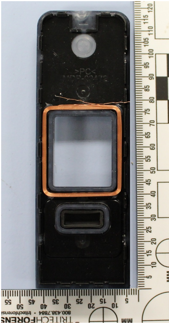
Model 20K (pigtail version) rear cover antenna
