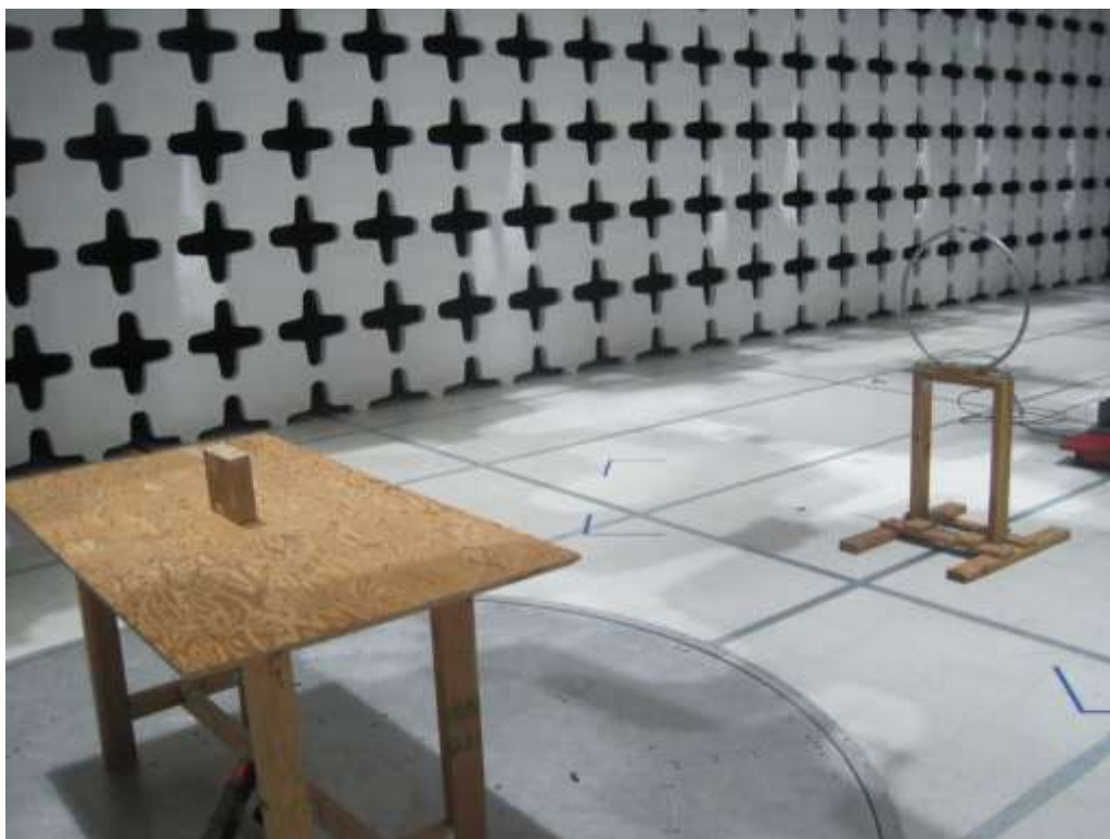
Radiated Emission<30MHz Test Setup – Rear View
