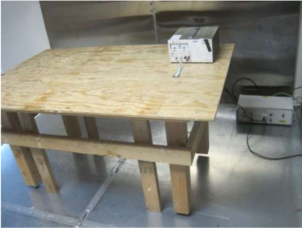
Conducted Emission Test Setup – Front View
