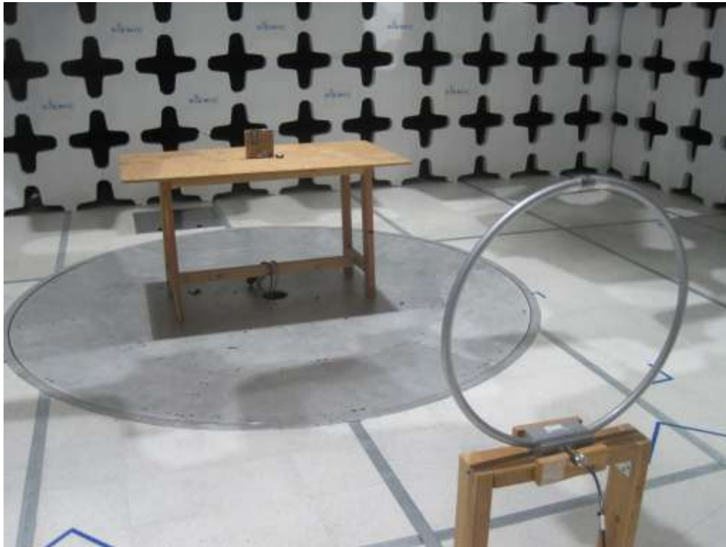
Radiated Emission<30MHz Test Setup – Front View
