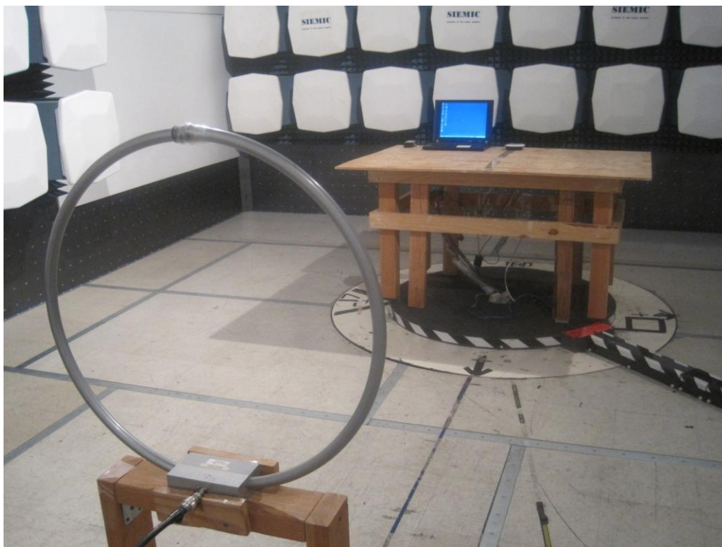
Radiated Emission (<30 MHz) – Front View
