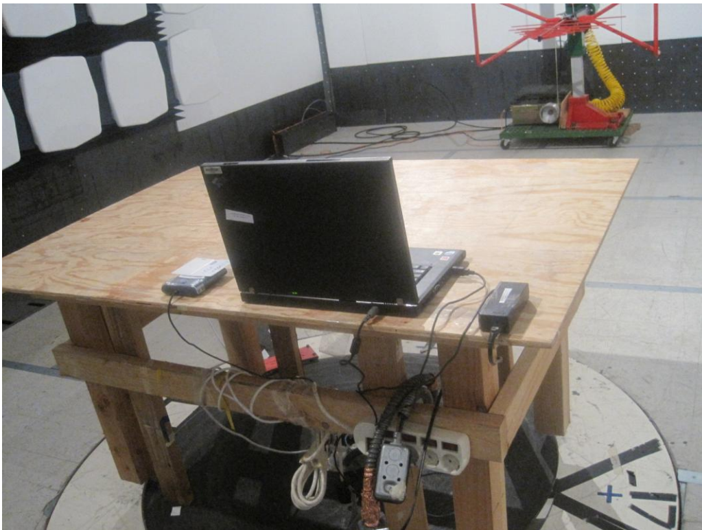
Radiated Emission (30 MHz – 1GHz) – Back View
