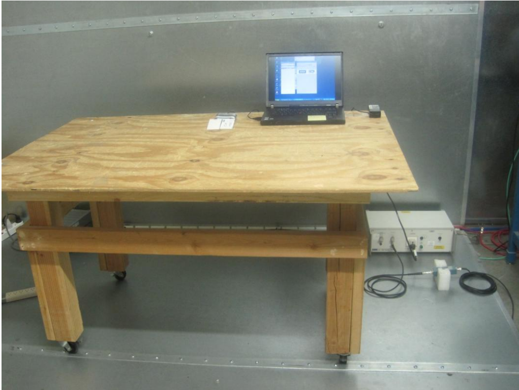
AC Line Conducted Emission - Front View
