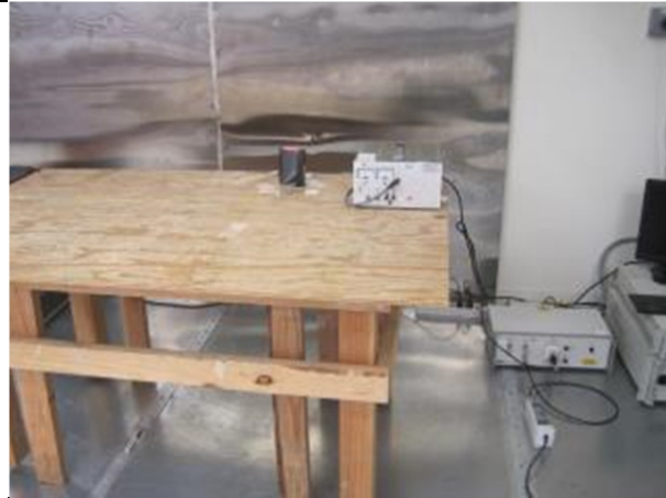
Conducted Emissions Test setup – Front View
