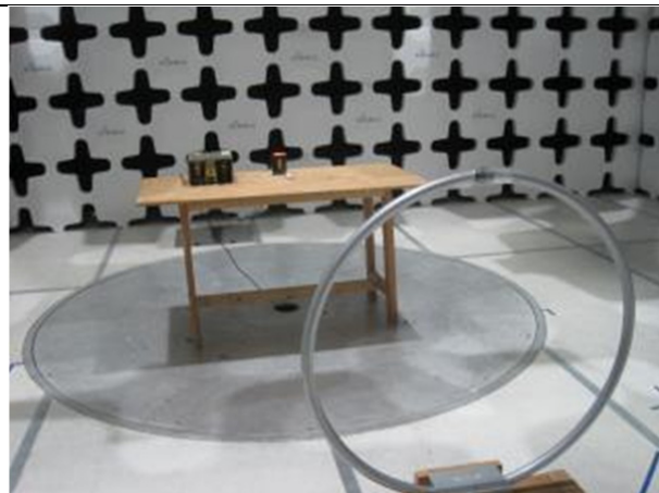
Radiated Emissions Test setup (<30MHz) – Front View
