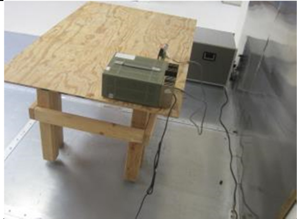
Conducted Emissions Test setup – Rear View
