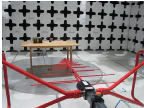
Radiated Emissions Test setup (<1GHz) – Front View
