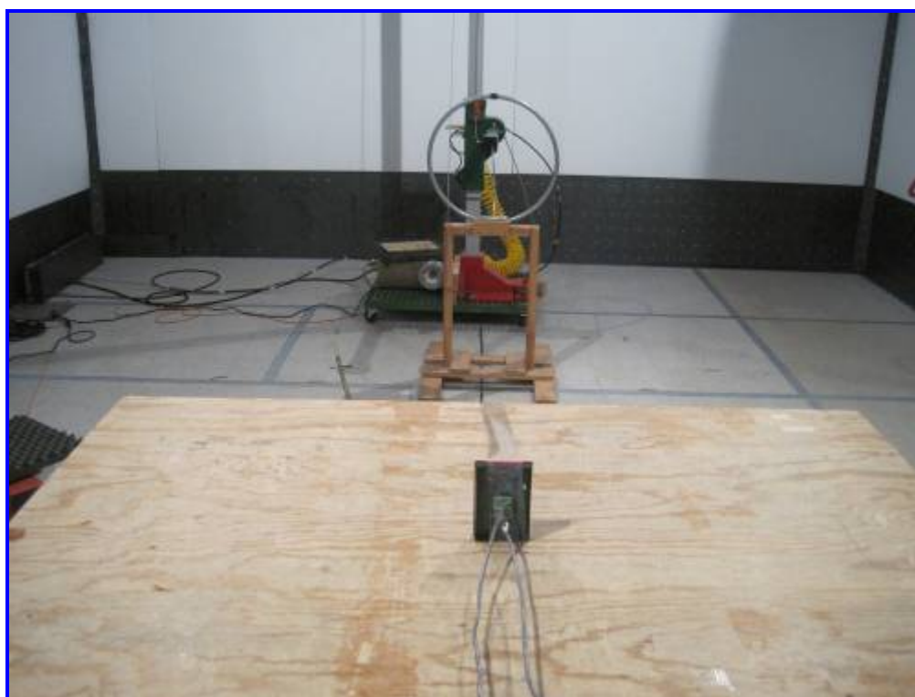
Radiated Emission (<30MHz) – Rear View
