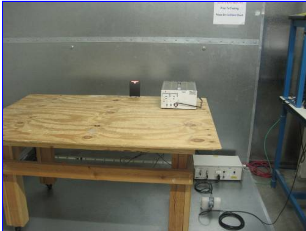
DC Line Conducted Emission - Front View
