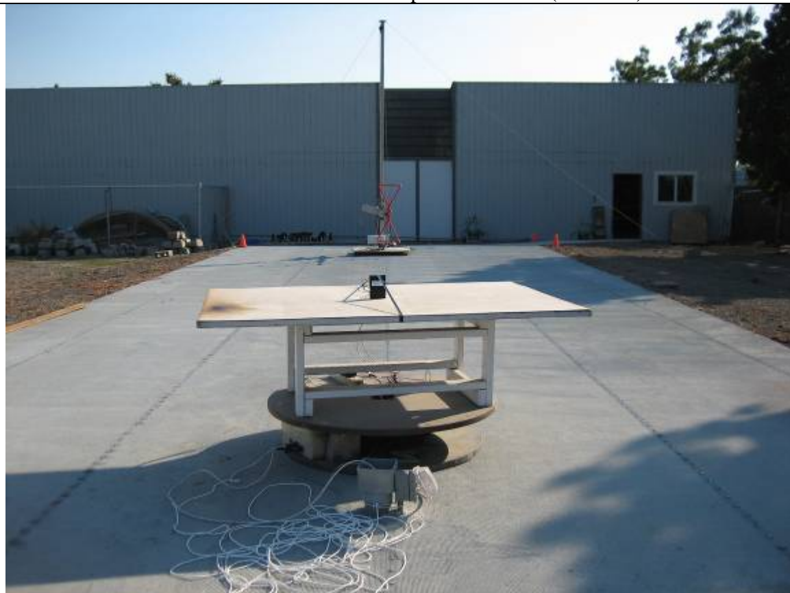
Radiated Emission Test Setup – Rear View ( >30\text{MHz} )
