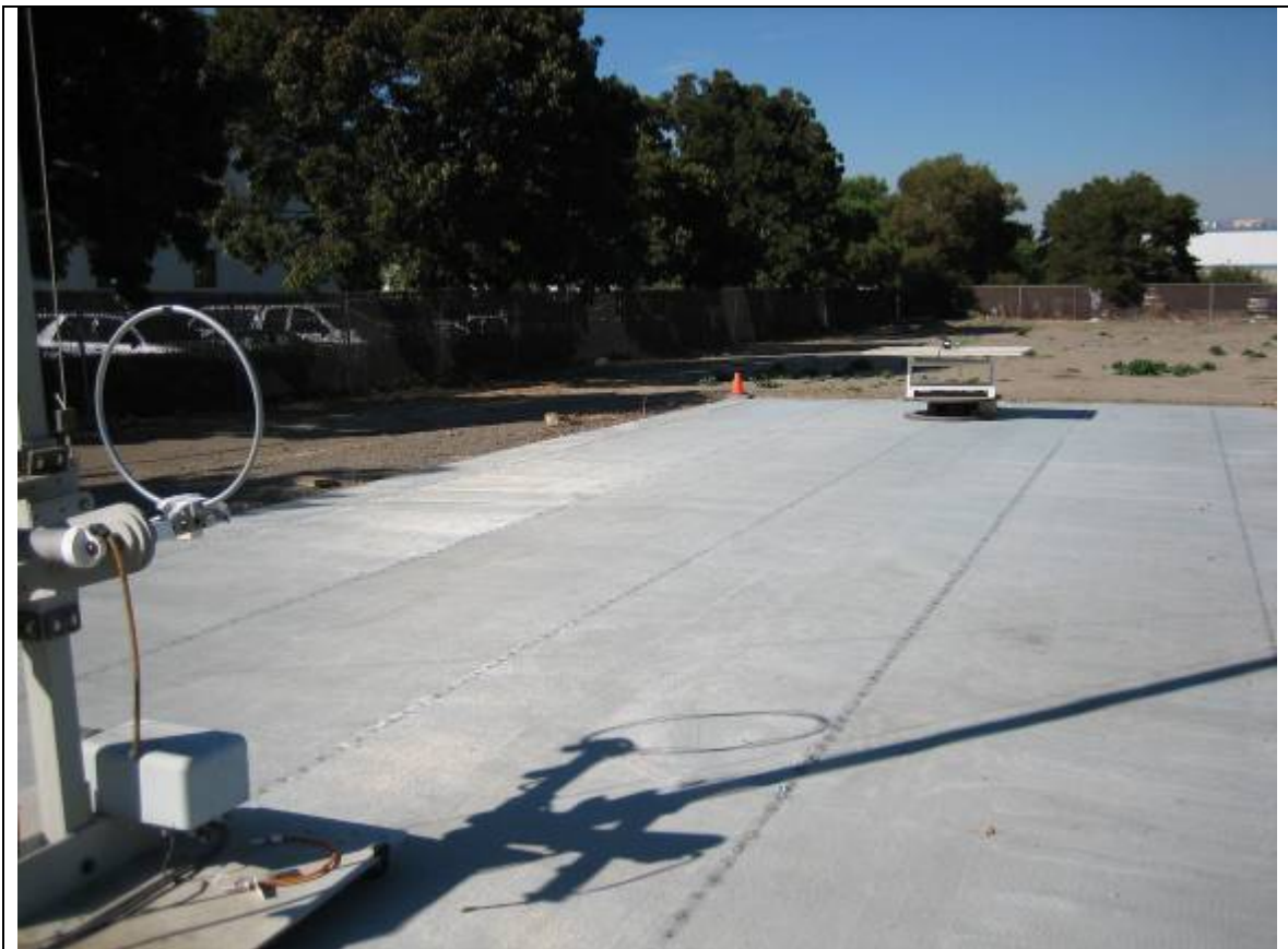
Radiated Emission Test Setup – Front View (<30MHz)
