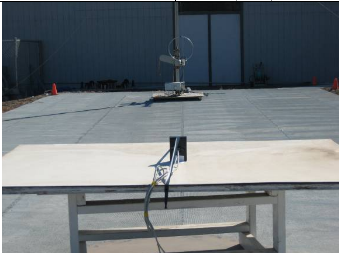
Radiated Emission Test Setup – Rear View (<30MHz)
