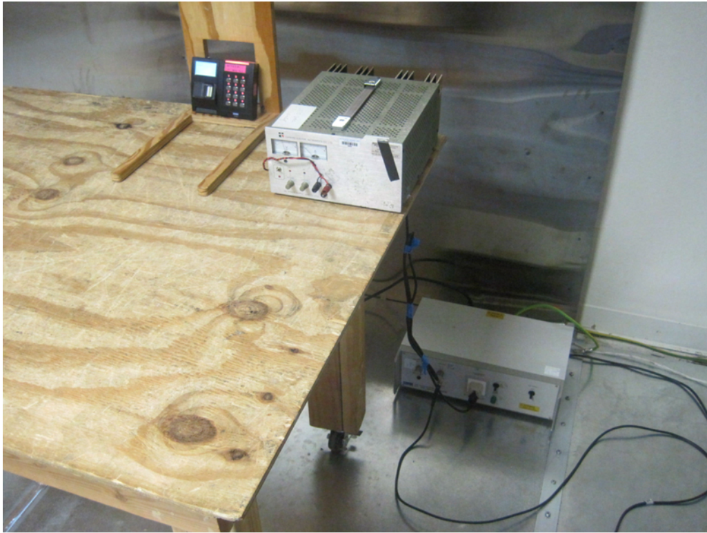
Conducted Emission Test Setup – Front View
