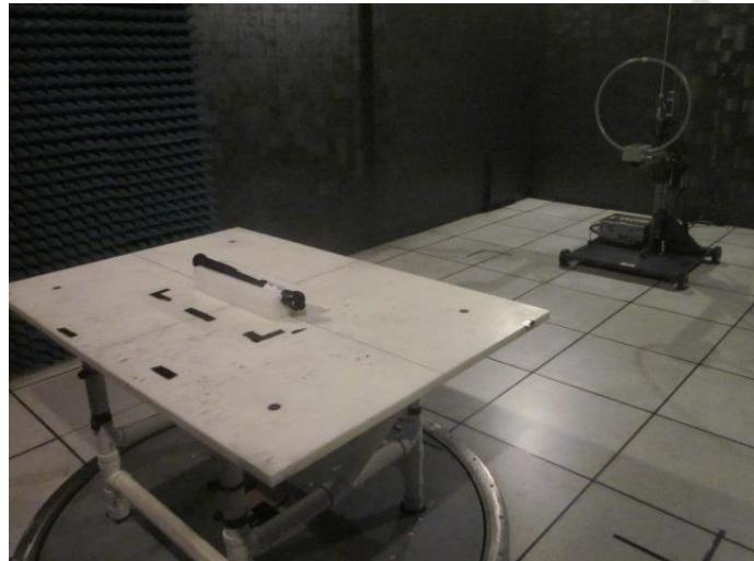
**30 MHz - 1000 MHz Radiated Emission**
