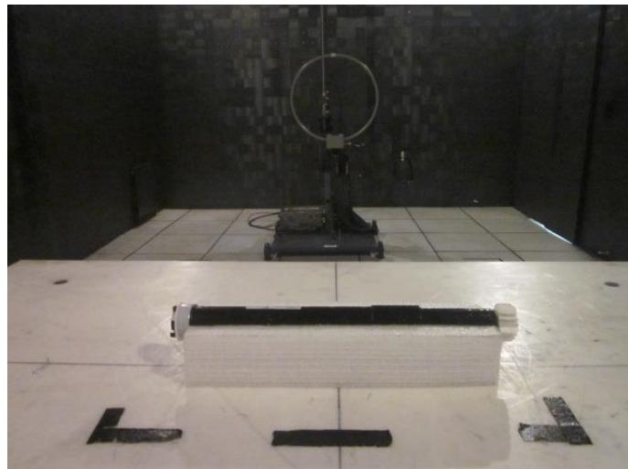
**30 MHz - 1000 MHz Radiated Emission**
