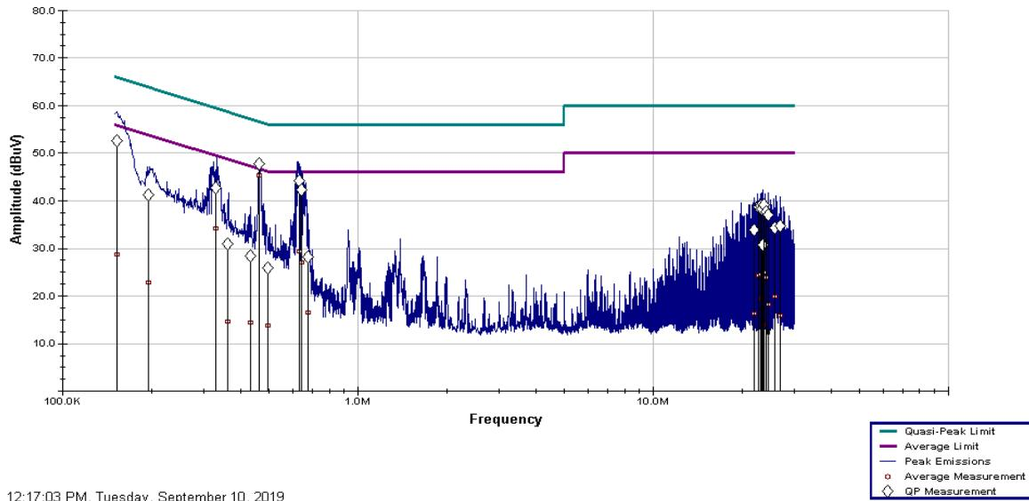
**Test Results:** Conducted emissions, from the Lutron Model KL01 Wireless Controlled LED Lamp, in transmit mode, comply with the requirements of 47 CFR Part 15.207 and RSS-Gen Section 8.7 for restricted bands of operation with a margin of 1.69 dB.
