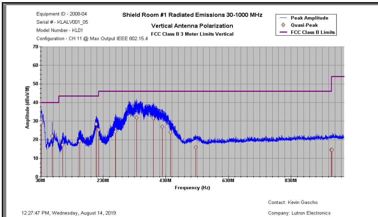
**Test Results:** Spurious radiated emissions, recorded at a distance of 3 meters from the Lutron Model KL01 Wireless Controlled LED Lamp, are below the 3-meter limit specified by FCC Section 15.209 and RSS-Gen Section 8.10 requirements by a margin of at least 6.41 dB.
