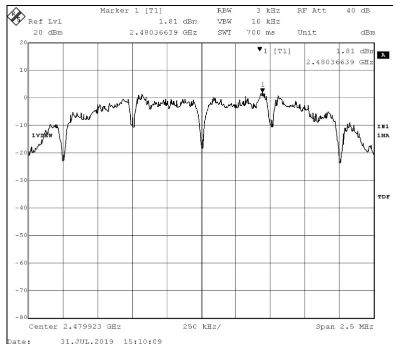
**Test Results:** The IEEE 802.15.4, Power Spectral Density measurements of the Lutron Model KL01 Wireless Controlled LED Lamp are compliant with the limits specified in FCC Section 15.247(e) and RSS-247 Section 5.2(b).
