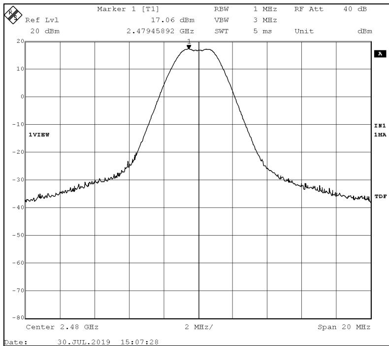
**Test Results:** The Peak Power Output measurements, with IEEE 802.15.4, OQPSK modulation, for the Lutron Model KL01 Wireless Controlled LED Lamp are compliant with the limits specified in FCC Section 15.247(b)(3).
