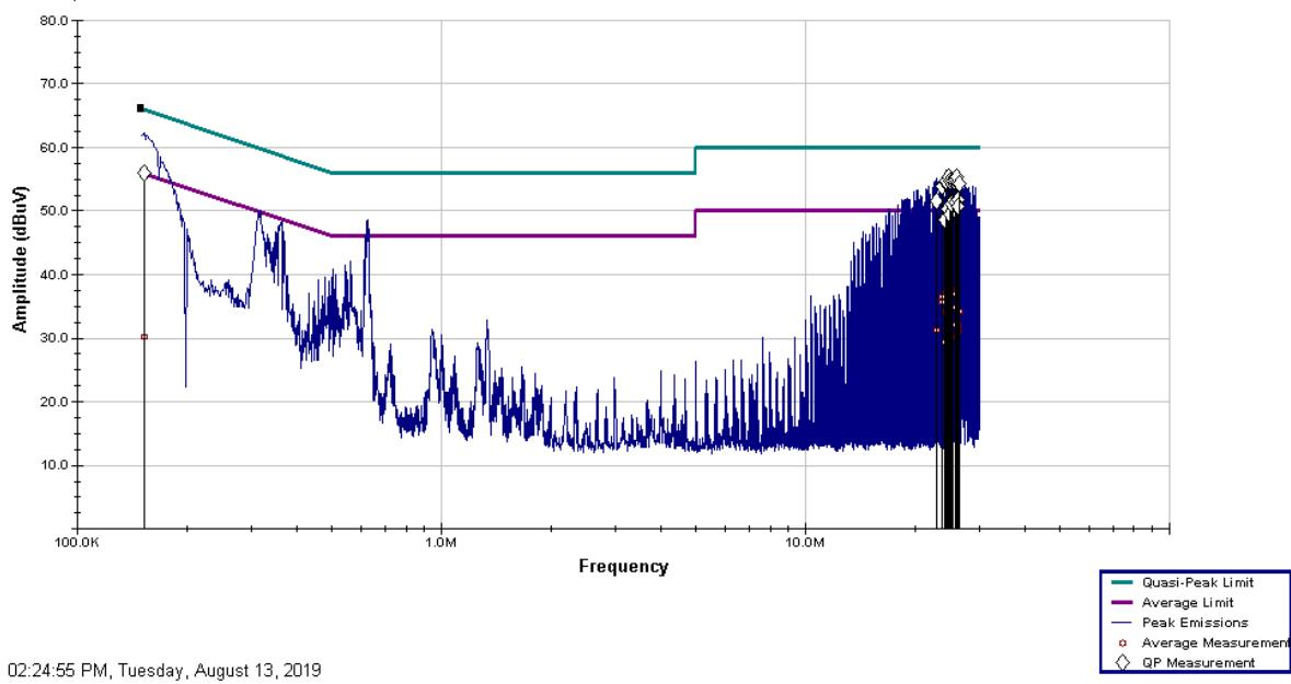
**Test Results:** Conducted emissions, from the Lutron Model KL01 Wireless Controlled LED Lamp, in receive mode, comply with the requirements of 47 CFR Part 15.207 and RSS-Gen Section 8.7 for restricted bands of operation with a margin of 4.58 dB.
