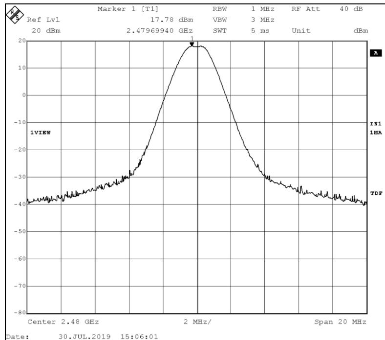
**Test Results:** The Peak Power Output measurements, with BLE, 2FSK modulation, for the Lutron Model KL01 Wireless Controlled LED Lamp are compliant with the limits specified in FCC Section 15.247(b)(3) and RSS-247 Section 5.4(d).
