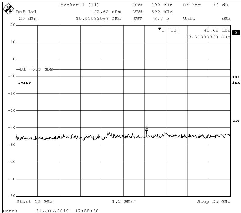
**Test Results:** The Antenna Conducted Spurious Emissions of the Lutron Model KL01 Wireless Controlled LED Lamp, operating with IEEE 802.15.4, OQPSK modulation are below the carrier -20 dB limit and therefore compliant with the limits specified in FCC Section 15.247(d).
