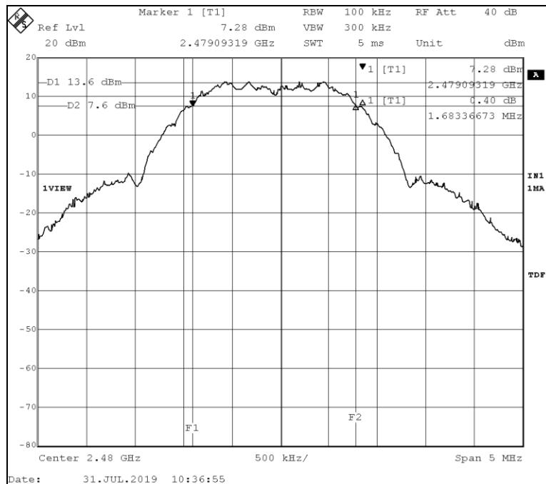
**Test Results:** The 6 dB, DTS Bandwidth measurements for the Lutron Model KL01 Wireless Controlled LED Lamp are compliant to 47 CFR Section 15.247(a)(2) and RSS-247 requirements of 500 kHz minimum.
