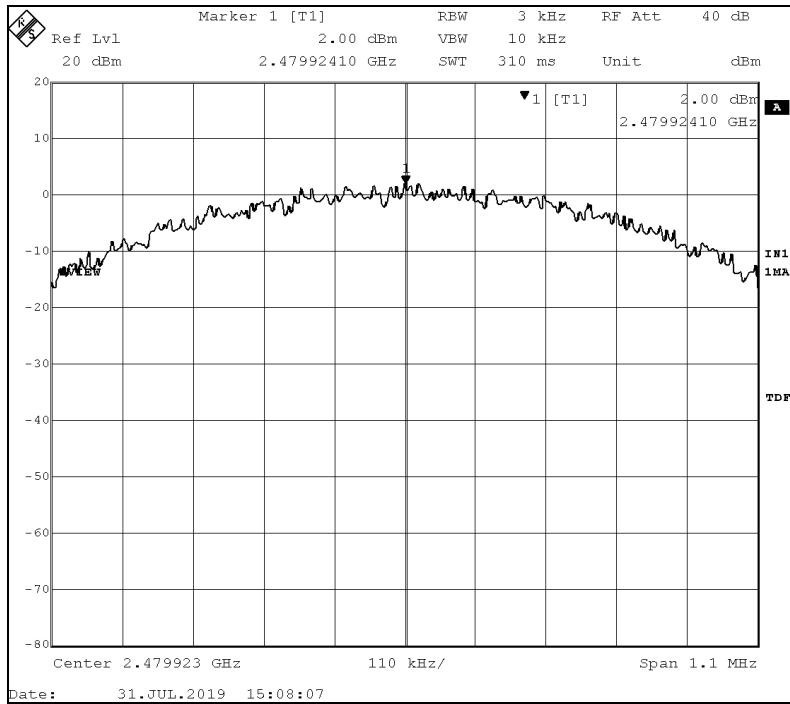
**Test Results:** The Power Spectral Density measurements of the Lutron Model KL01 Wireless Controlled LED Lamp are compliant with the limits specified in FCC Section 15.247(e) and RSS-247 Section 5.2(b).
