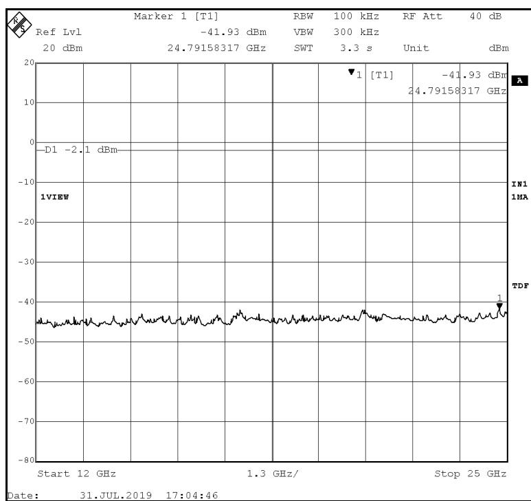
**Test Results:** The Antenna Conducted Spurious Emissions of the Lutron Model KL01 Wireless Controlled LED Lamp, operating with BLE, 2FSK modulation are below the carrier –20 dB limit and therefore compliant with the limits specified in FCC Section 15.247(d).
