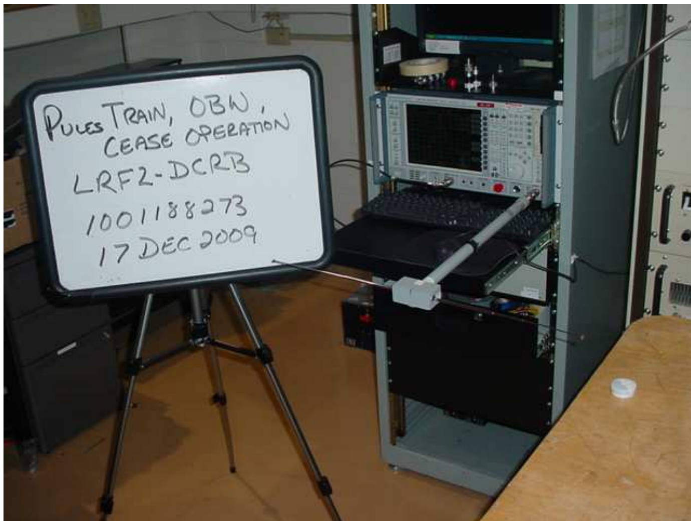
Figure 1 Test Setup for Occupied Bandwidth
