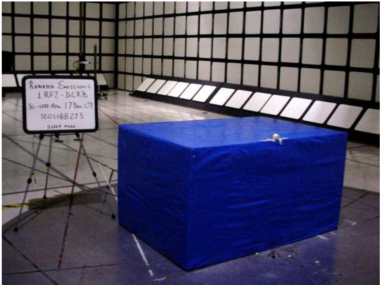
Figure 15 Test setup for Radiated Emissions
