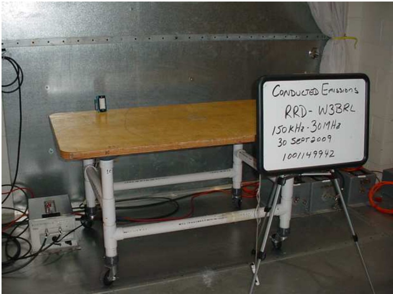
Figure 1 Test Setup for Conducted Emissions
