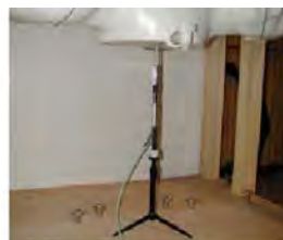
Figure 11.1 Dipole Verification Test Setup Diagram & Photo
