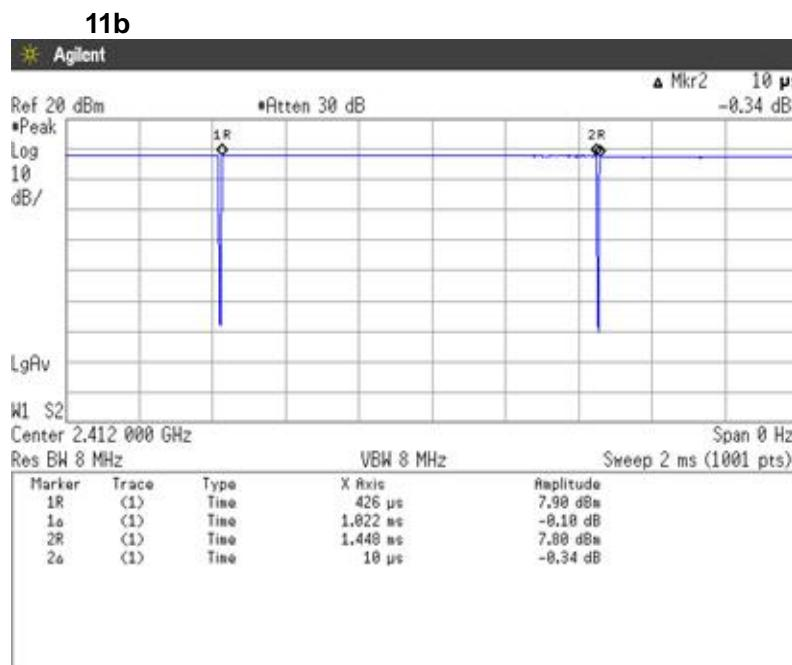
$$\text{Duty Cycle} = \text{Ton} / (\text{Ton} + \text{Toff}) = 1022[\mu\text{s}] / (1022[\mu\text{s}] + 10[\mu\text{s}]) = 99.03[\%]$$
