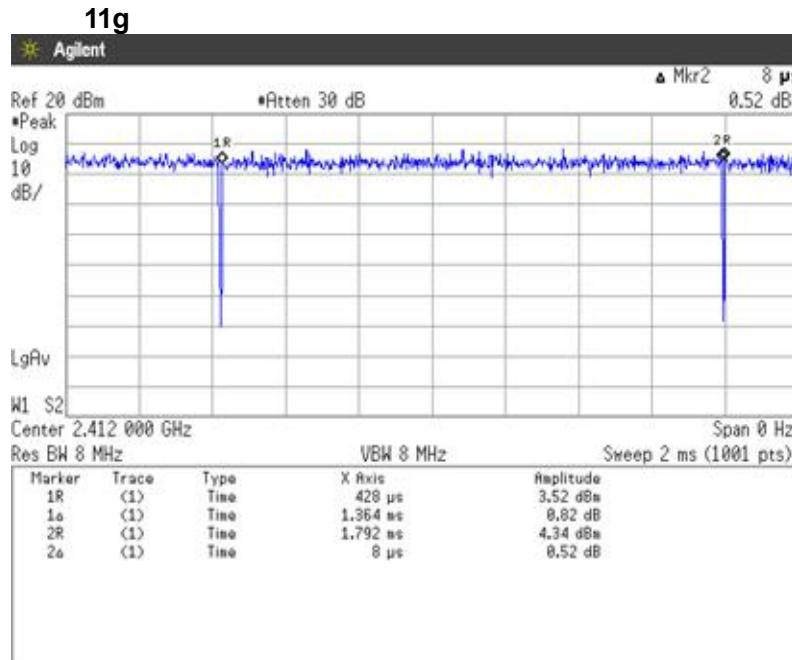
$$\text{Duty Cycle} = \text{Ton} / (\text{Ton} + \text{Toff}) = 1364[\mu\text{s}] / (1364[\mu\text{s}] + 8[\mu\text{s}]) = 99.42[\%]$$
