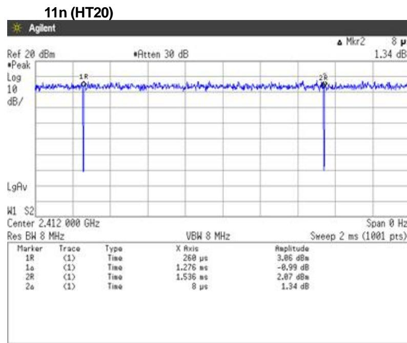
Duty Cycle = Ton / (Ton + Toff) = 1276[μs] / (1276[μs] + 8[μs]) = 99.38[%]
