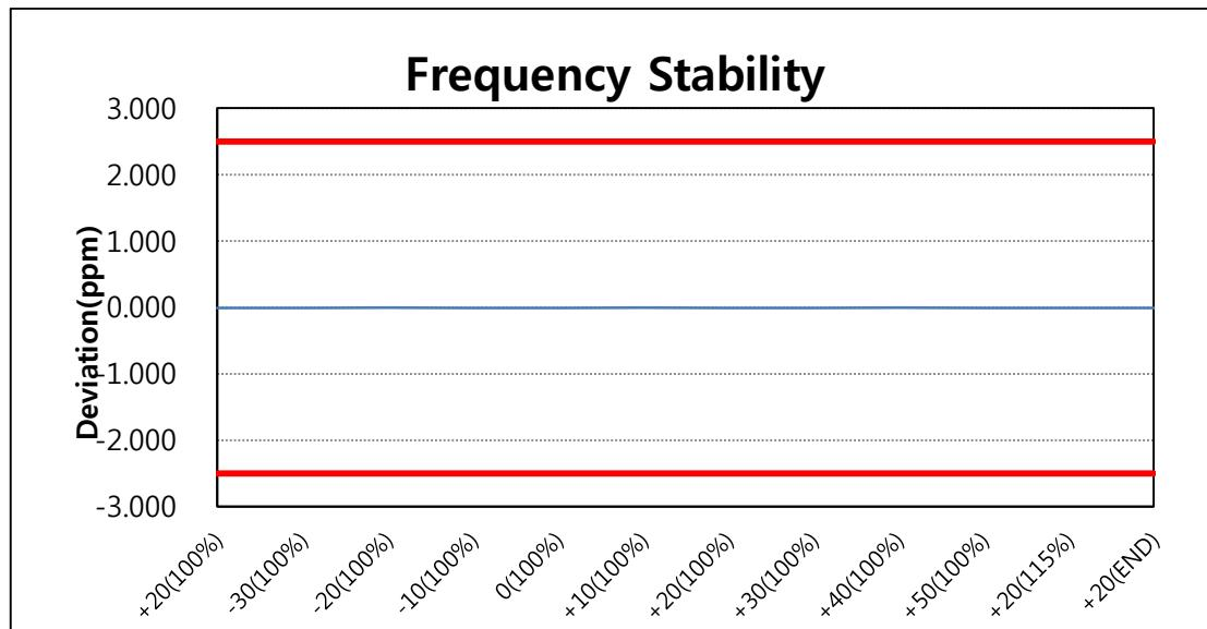
**Note.** Based on the results of the frequency stability test at the center channel the frequency deviation results measured are very small. as such it is determined that the channels at the band edge would remain inband when the maximum measured frequency deviation noted during the frequency stability tests is applied. therefore the device is determined to remain operating in band over the temperature and voltage range as tested.
