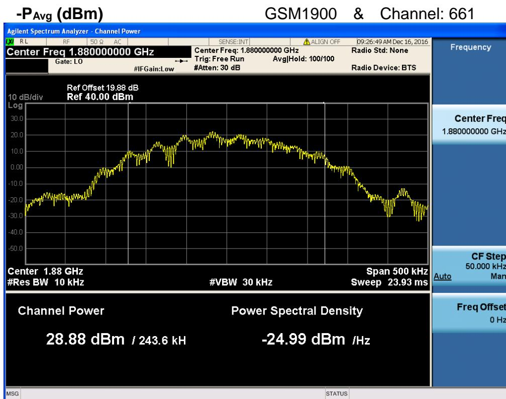
$$\text{PAPR (dB)} = \text{P}_{\text{Pk}} (\text{dBm}) - \text{P}_{\text{Avg}} (\text{dBm}) = 29.23 \text{ dBm} - 28.88 \text{ dBm} = 0.35 \text{ dB}$$
