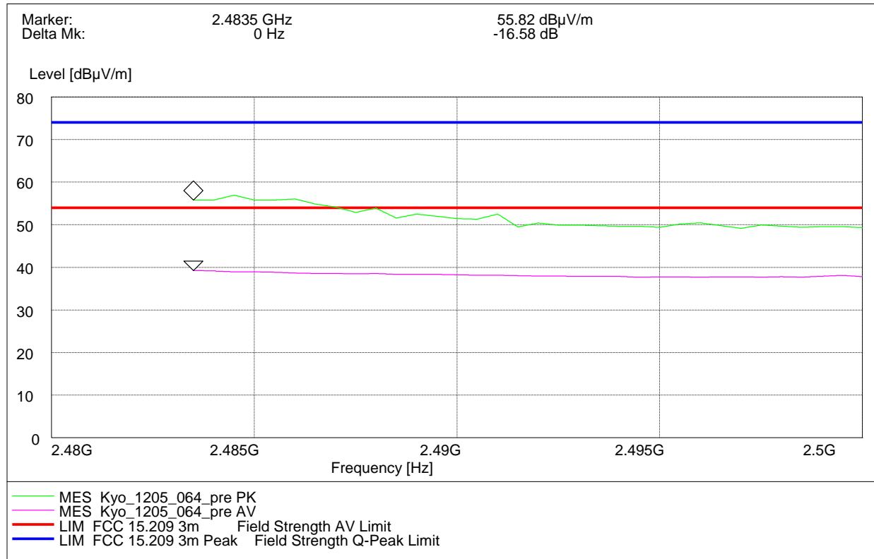
Radiated measurement (higher band edge)
