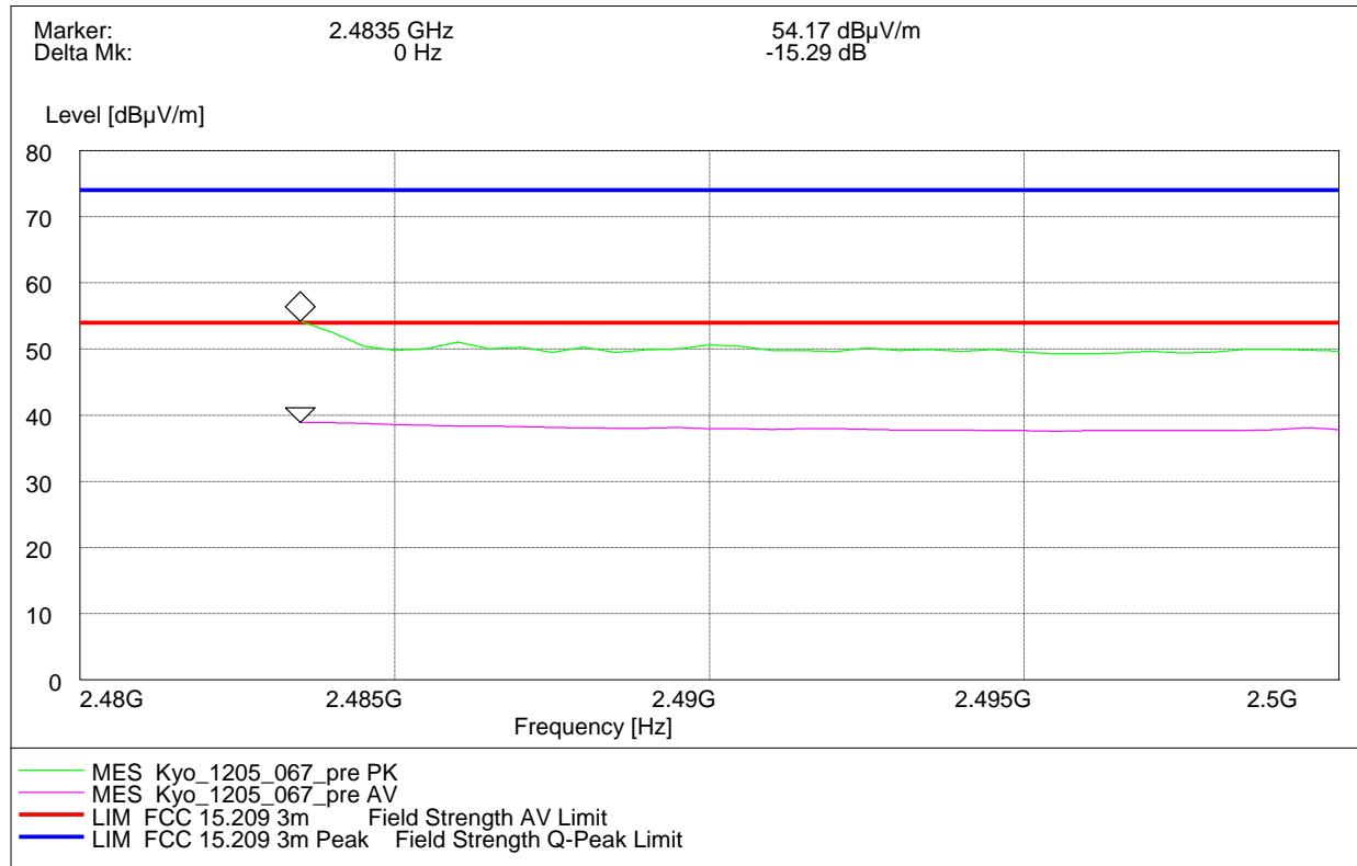
Radiated measurement (higher band edge)
