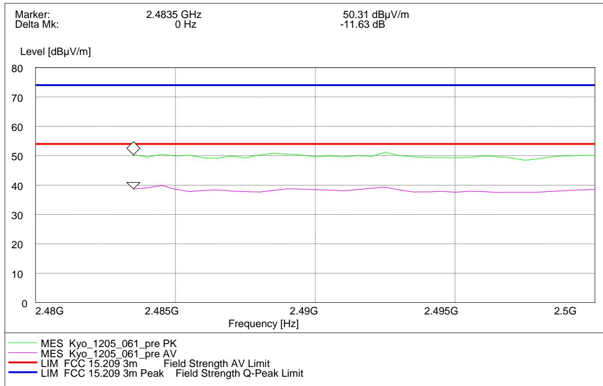
Radiated measurement (higher band edge)
