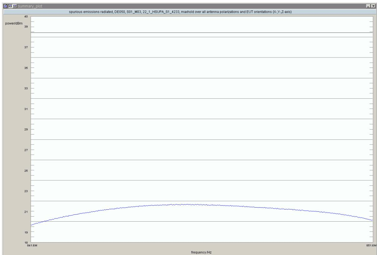
**Test: 22.1; Frequency Band = FDD5, Mode = HSUPA\_subtest\_2, Channel = 4132, Frequency = 826.4MHz, Method = conducted**
