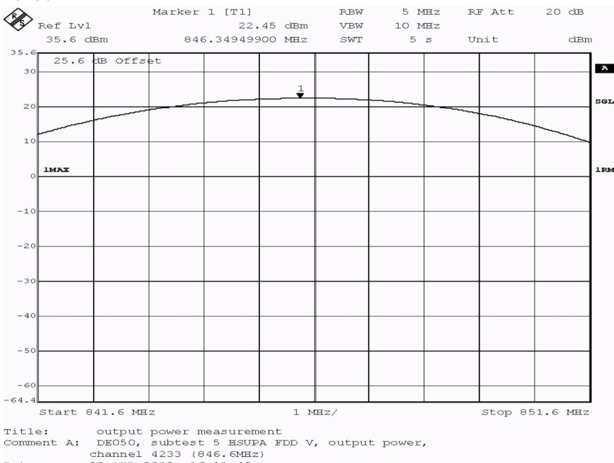
**Test: 22.1; Frequency Band = FDD5, Mode = HSUPA\_subtest\_5, Channel = 4233, Frequency = 846.6MHz, Method = radiated**
