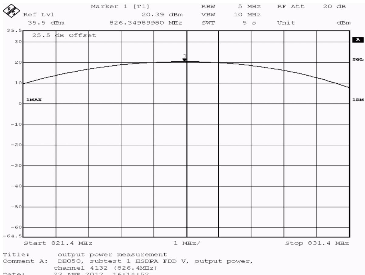
**Test: 22.1; Frequency Band = FDD5, Mode = HSDPA\_subtest\_1, Channel = 4132, Frequency = 826.4MHz, Method = radiated**
