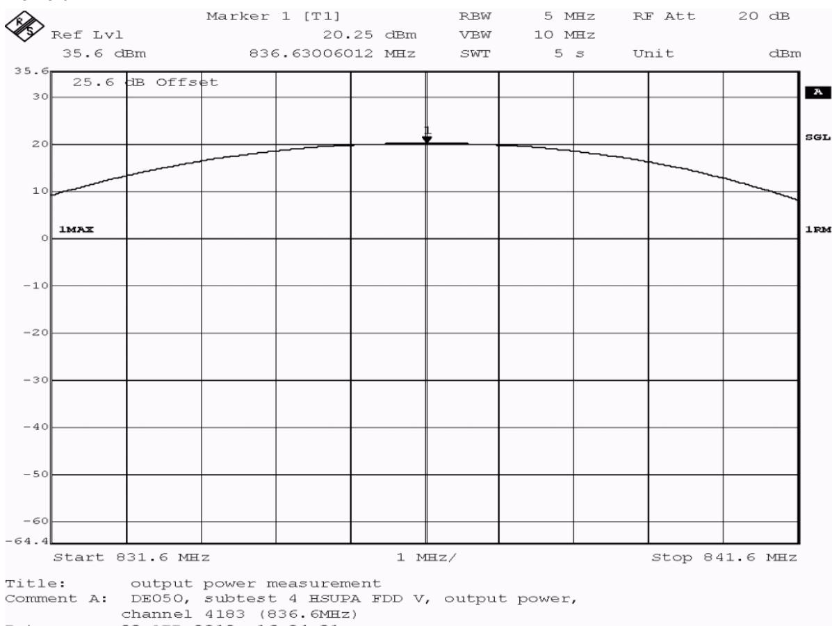
**Test: 22.1; Frequency Band = FDD5, Mode = HSUPA\_subtest\_4, Channel = 4183, Frequency = 836.6MHz, Method = radiated**
