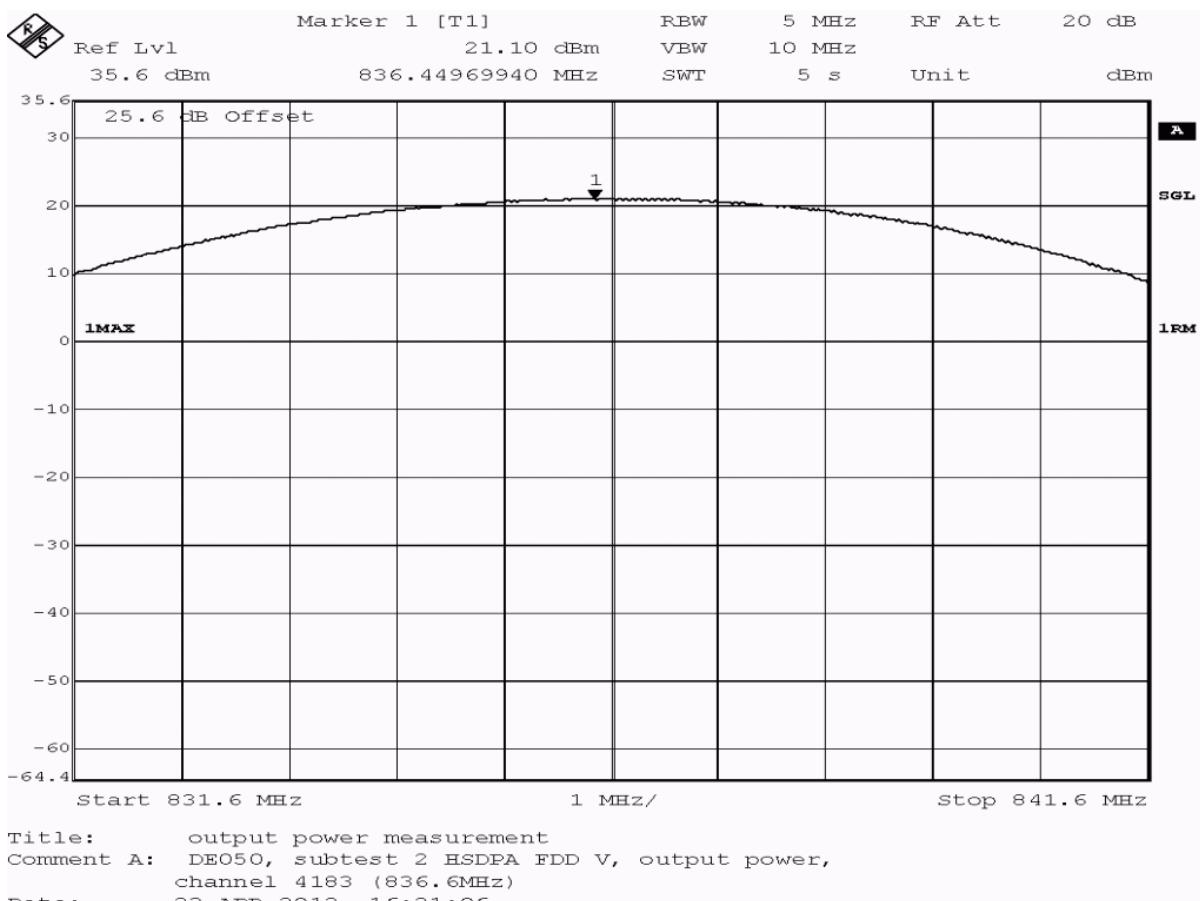
**Test: 22.1; Frequency Band = FDD5, Mode = HSDPA\_subtest\_2, Channel = 4183, Frequency = 836.6MHz, Method = radiated**
