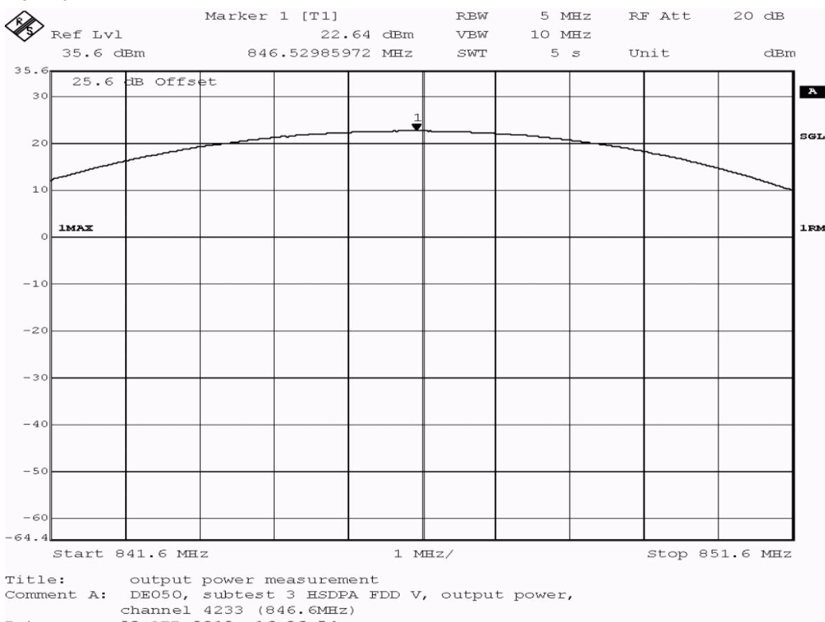
**Test: 22.1; Frequency Band = FDD5, Mode = HSDPA\_subtest\_3, Channel = 4233, Frequency = 846.6MHz, Method = radiated**
