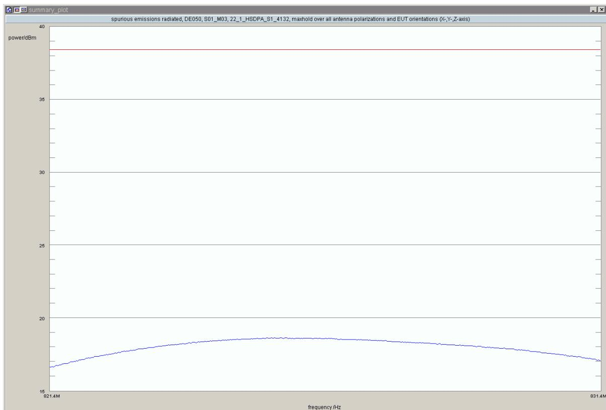
**Test: 22.1; Frequency Band = FDD5, Mode = HSDPA\_subtest\_1, Channel = 4183, Frequency = 836.6MHz, Method = conducted**
