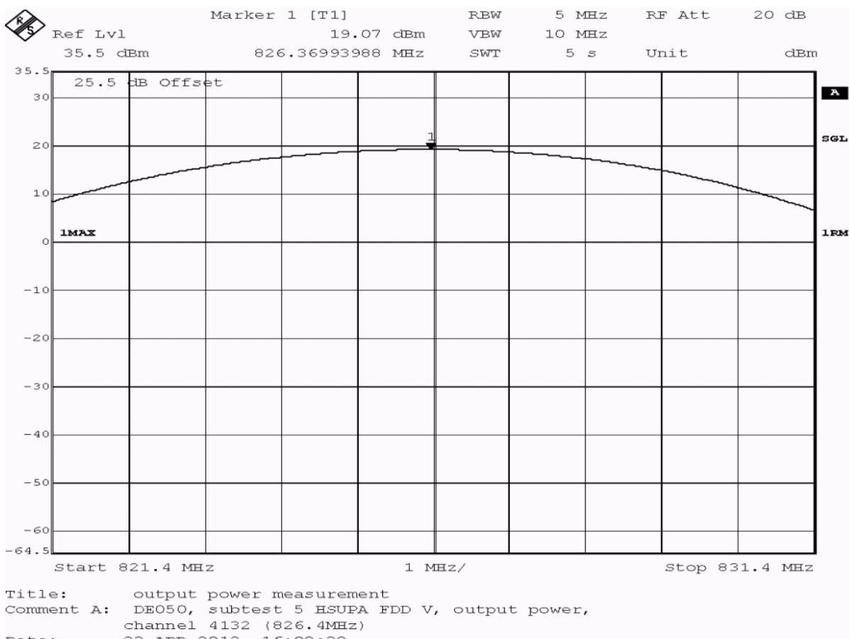
**Test: 22.1; Frequency Band = FDD5, Mode = HSUPA\_subtest\_5, Channel = 4132, Frequency = 826.4MHz, Method = radiated**
