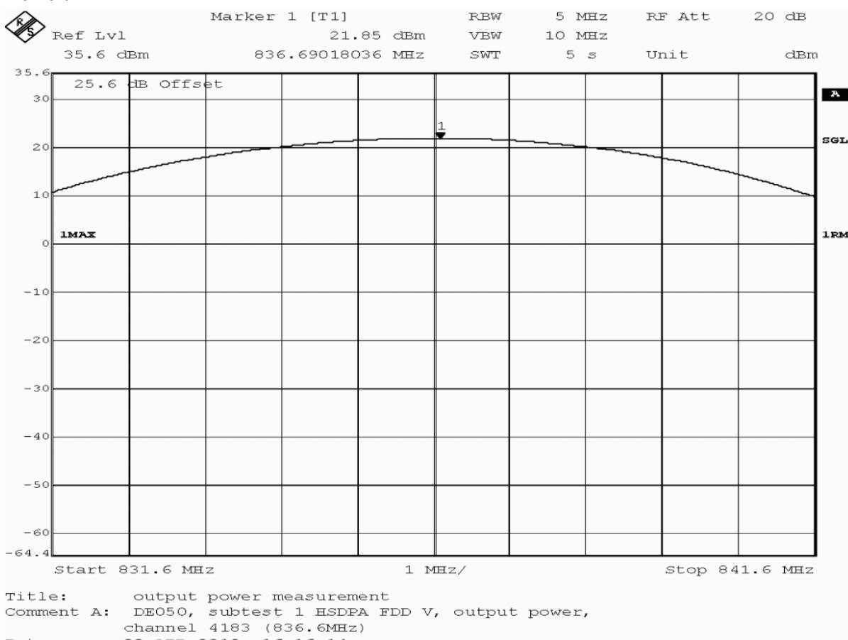
**Test: 22.1; Frequency Band = FDD5, Mode = HSDPA\_subtest\_1, Channel = 4183, Frequency = 836.6MHz, Method = radiated**
