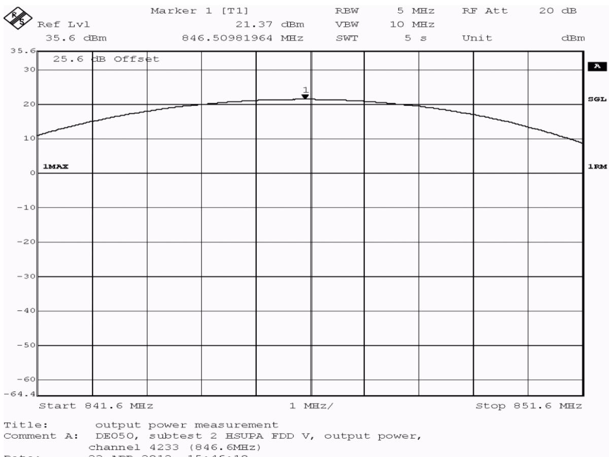
**Test: 22.1; Frequency Band = FDD5, Mode = HSUPA\_subtest\_2, Channel = 4233, Frequency = 846.6MHz, Method = radiated**
