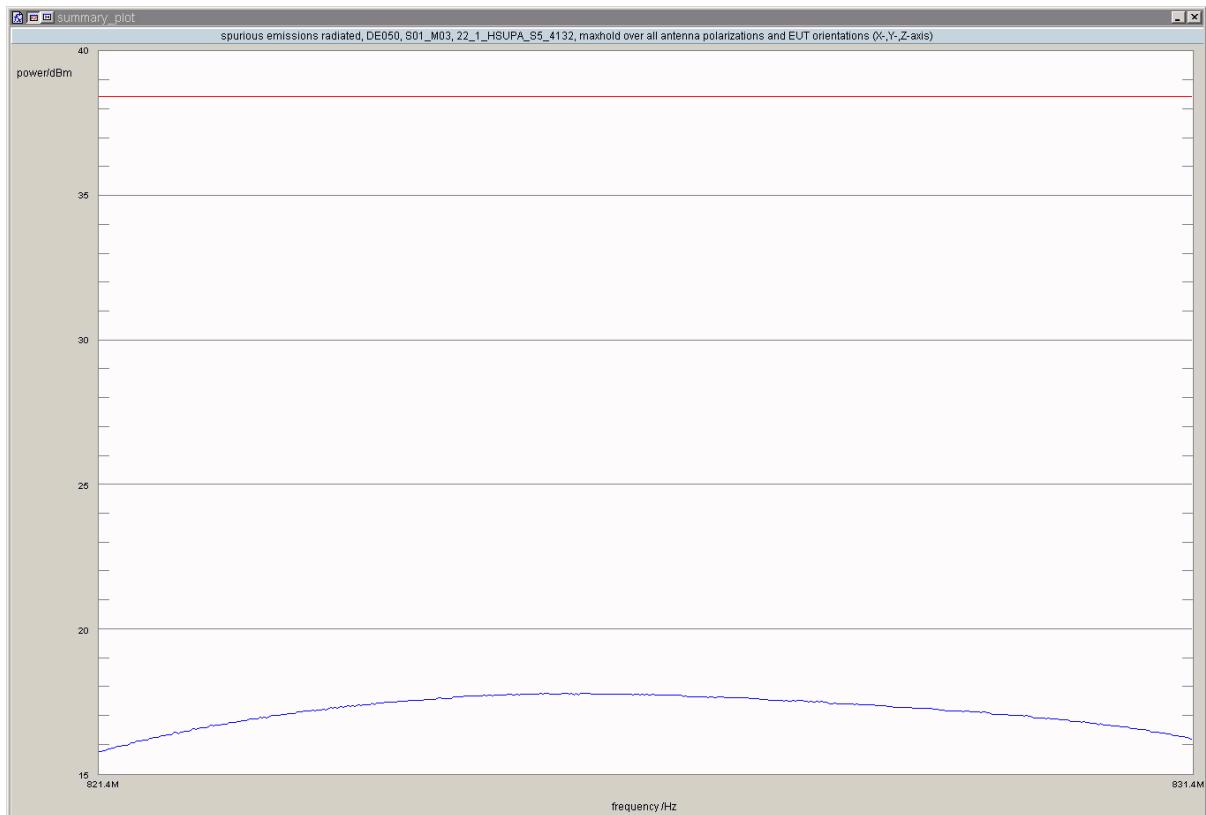
**Test: 22.1; Frequency Band = FDD5, Mode = HSUPA\_subtest\_5, Channel = 4183, Frequency = 836.6MHz, Method = conducted**
