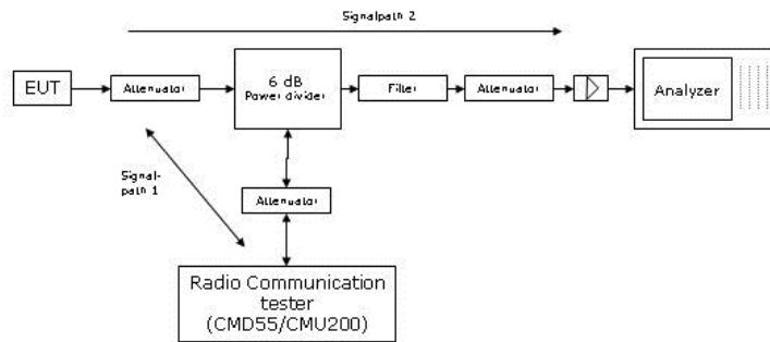
Remark: Depending on the frequency range suitable attenuators and/or filters and/or amplifiers are used.
