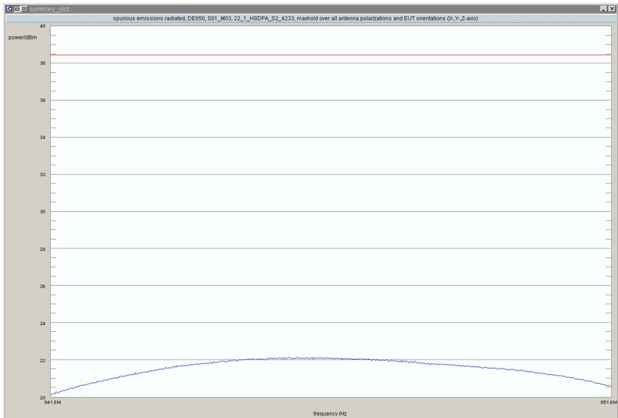
**Test: 22.1; Frequency Band = FDD5, Mode = HSDPA\_subtest\_3, Channel = 4132, Frequency = 826.4MHz, Method = conducted**
