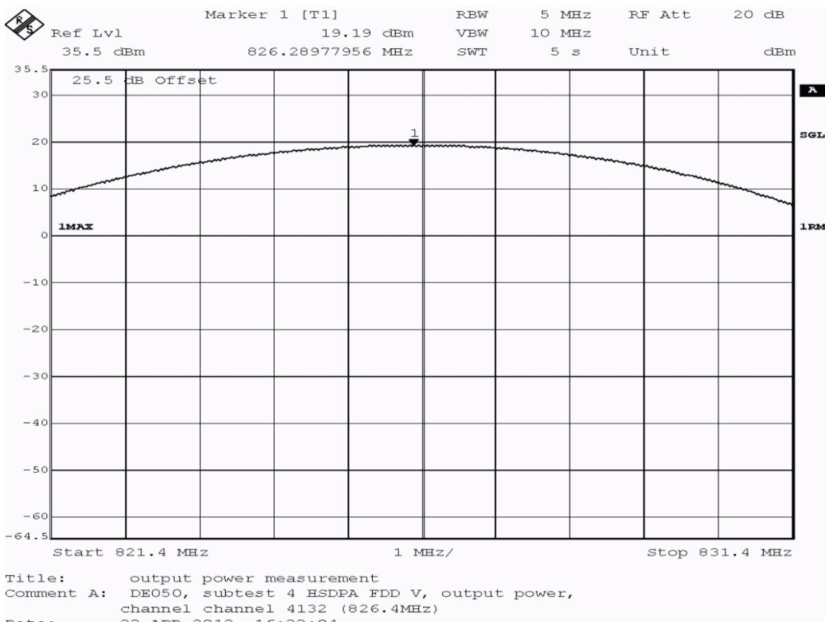
**Test: 22.1; Frequency Band = FDD5, Mode = HSDPA\_subtest\_4, Channel = 4132, Frequency = 826.4MHz, Method = radiated**
