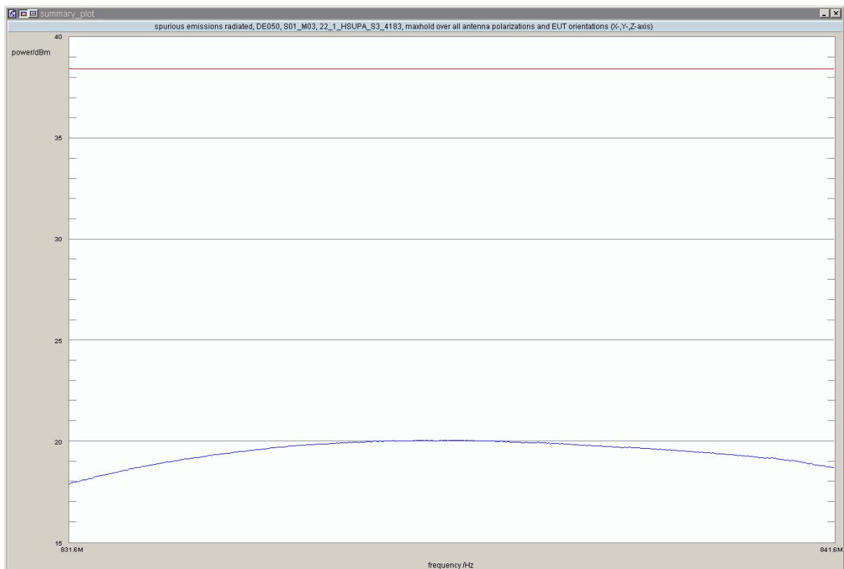
**Test: 22.1; Frequency Band = FDD5, Mode = HSUPA\_subtest\_3, Channel = 4233, Frequency = 846.6MHz, Method = conducted**
