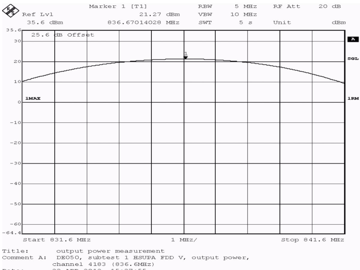
Test: 22.1; Frequency Band = FDD5, Mode = HSUPA\_subtest\_1, Channel = 4183, Frequency = 836.6MHz, Method = radiated
