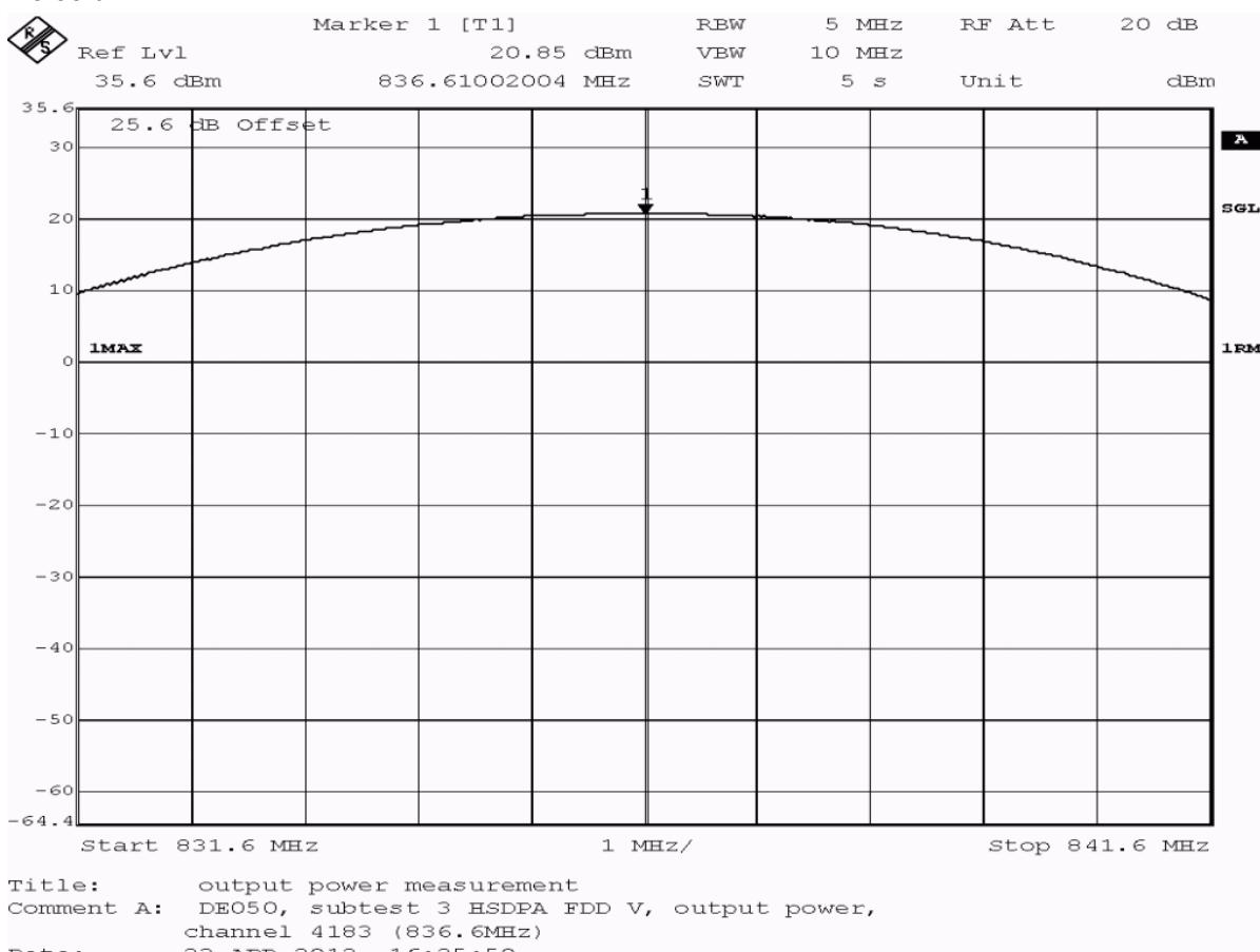
**Test: 22.1; Frequency Band = FDD5, Mode = HSDPA\_subtest\_3, Channel = 4183, Frequency = 836.6MHz, Method = radiated**
