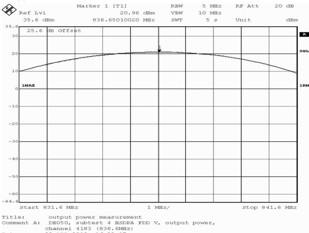
**Test: 22.1; Frequency Band = FDD5, Mode = HSDPA\_subtest\_4, Channel = 4183, Frequency = 836.6MHz, Method = radiated**
