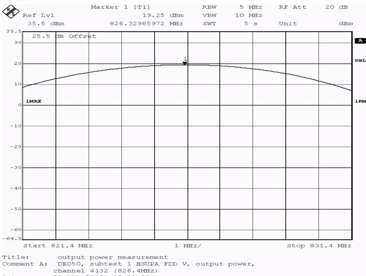
**Test: 22.1; Frequency Band = FDD5, Mode = HSUPA\_subtest\_1, Channel = 4132, Frequency = 826.4MHz, Method = radiated**
