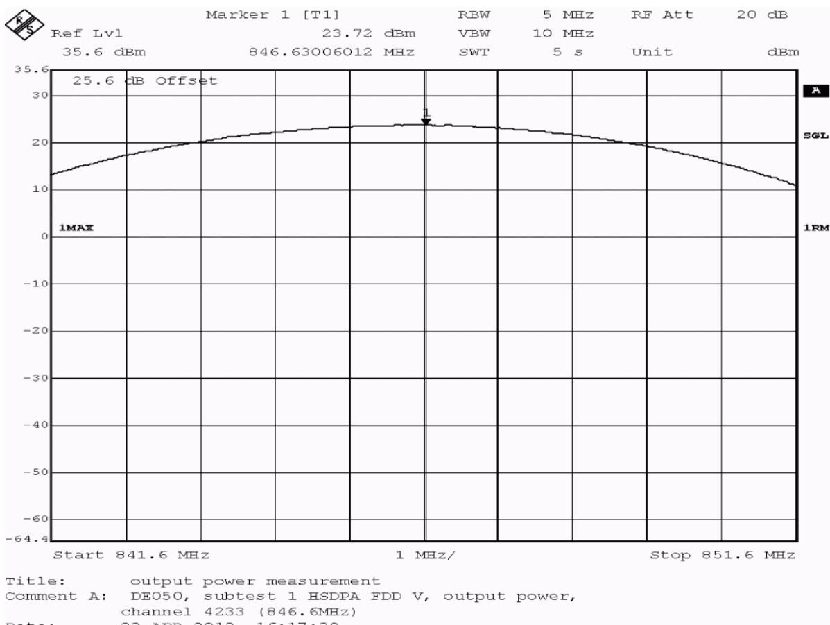
**Test: 22.1; Frequency Band = FDD5, Mode = HSDPA\_subtest\_1, Channel = 4233, Frequency = 846.6MHz, Method = radiated**
