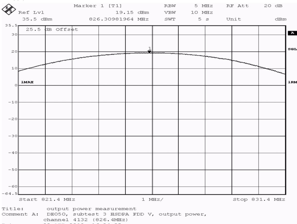
**Test: 22.1; Frequency Band = FDD5, Mode = HSDPA\_subtest\_3, Channel = 4132, Frequency = 826.4MHz, Method = radiated**
