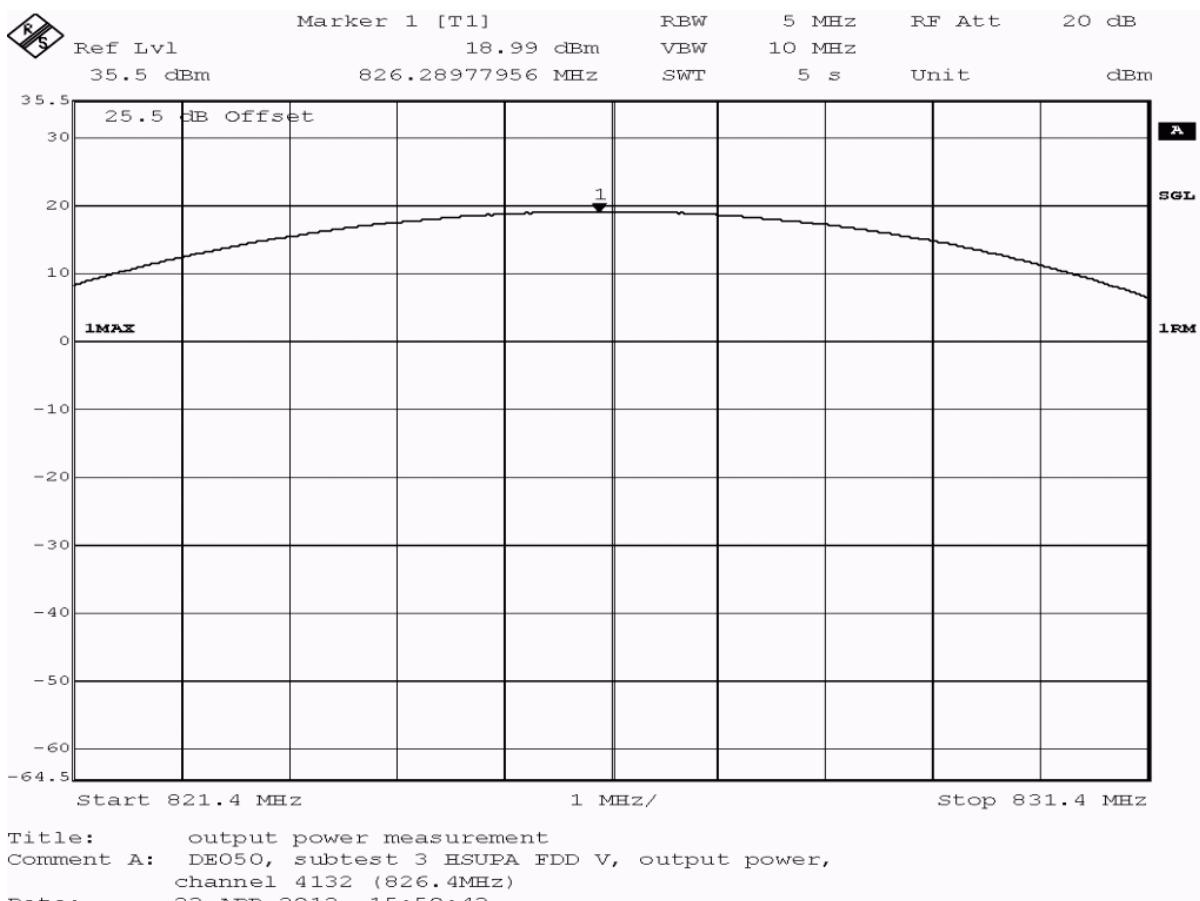
**Test: 22.1; Frequency Band = FDD5, Mode = HSUPA\_subtest\_3, Channel = 4132, Frequency = 826.4MHz, Method = radiated**
