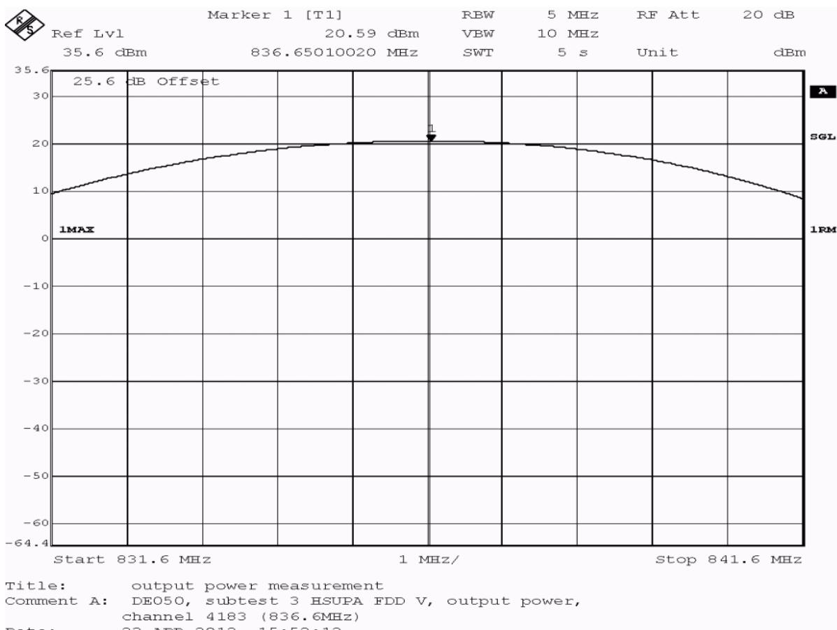
**Test: 22.1; Frequency Band = FDD5, Mode = HSUPA\_subtest\_3, Channel = 4183, Frequency = 836.6MHz, Method = radiated**
