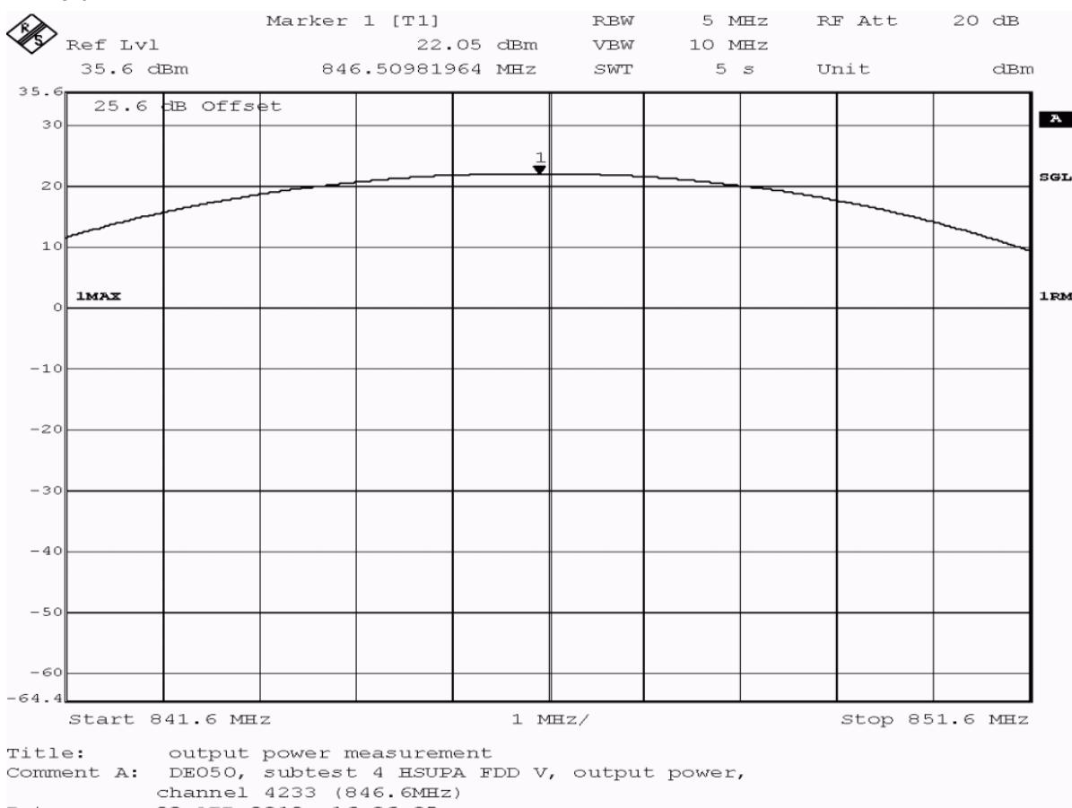
**Test: 22.1; Frequency Band = FDD5, Mode = HSUPA\_subtest\_4, Channel = 4233, Frequency = 846.6MHz, Method = radiated**
