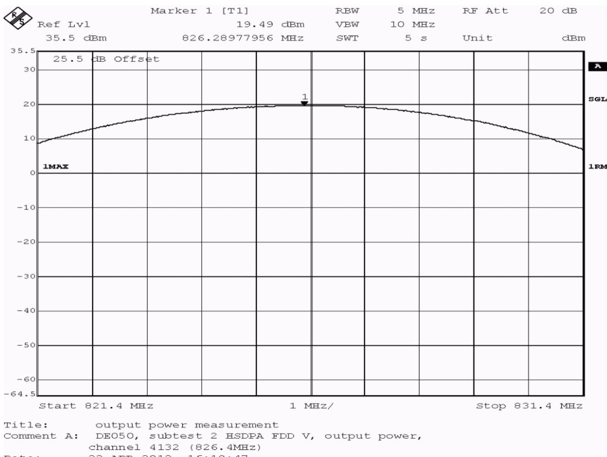
**Test: 22.1; Frequency Band = FDD5, Mode = HSDPA\_subtest\_2, Channel = 4132, Frequency = 826.4MHz, Method = radiated**
