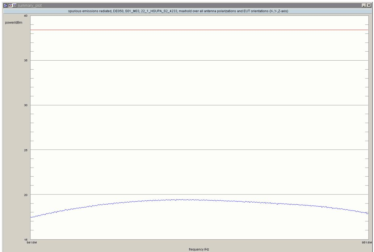
**Test: 22.1; Frequency Band = FDD5, Mode = HSUPA\_subtest\_3, Channel = 4132, Frequency = 826.4MHz, Method = conducted**
