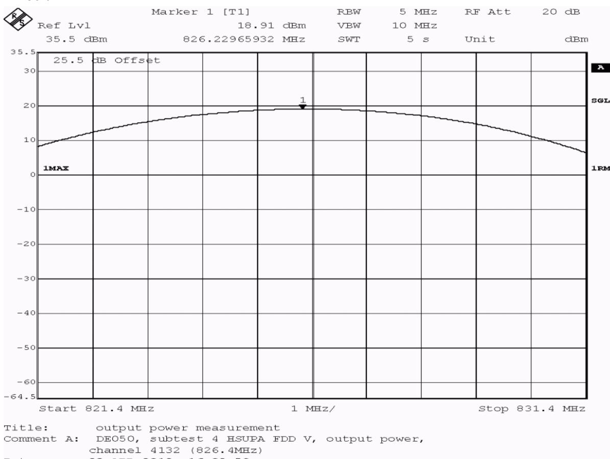
**Test: 22.1; Frequency Band = FDD5, Mode = HSUPA\_subtest\_4, Channel = 4132, Frequency = 826.4MHz, Method = radiated**
