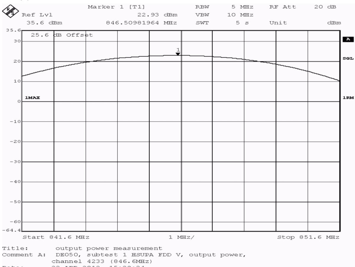
**Test: 22.1; Frequency Band = FDD5, Mode = HSUPA\_subtest\_1, Channel = 4233, Frequency = 846.6MHz, Method = radiated**
