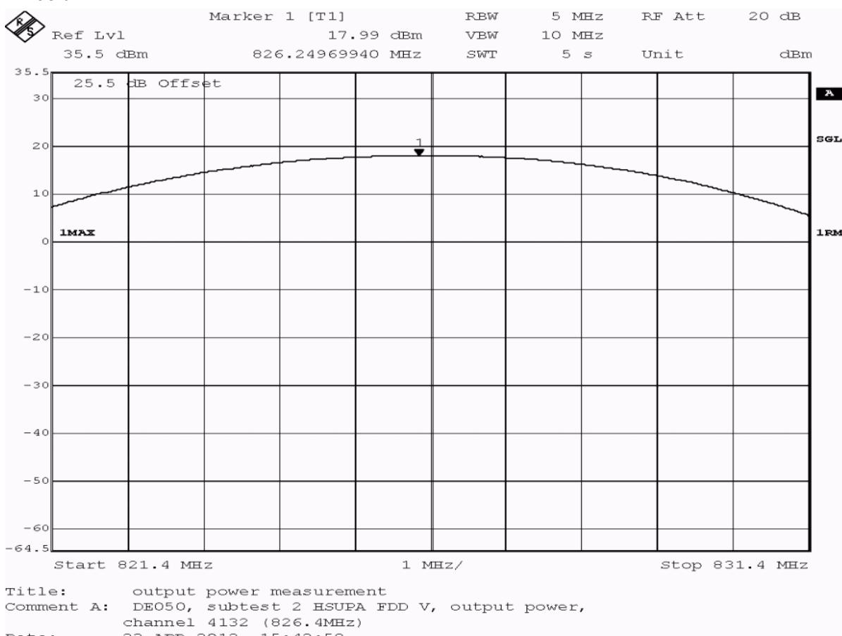
**Test: 22.1; Frequency Band = FDD5, Mode = HSUPA\_subtest\_2, Channel = 4132, Frequency = 826.4MHz, Method = radiated**
