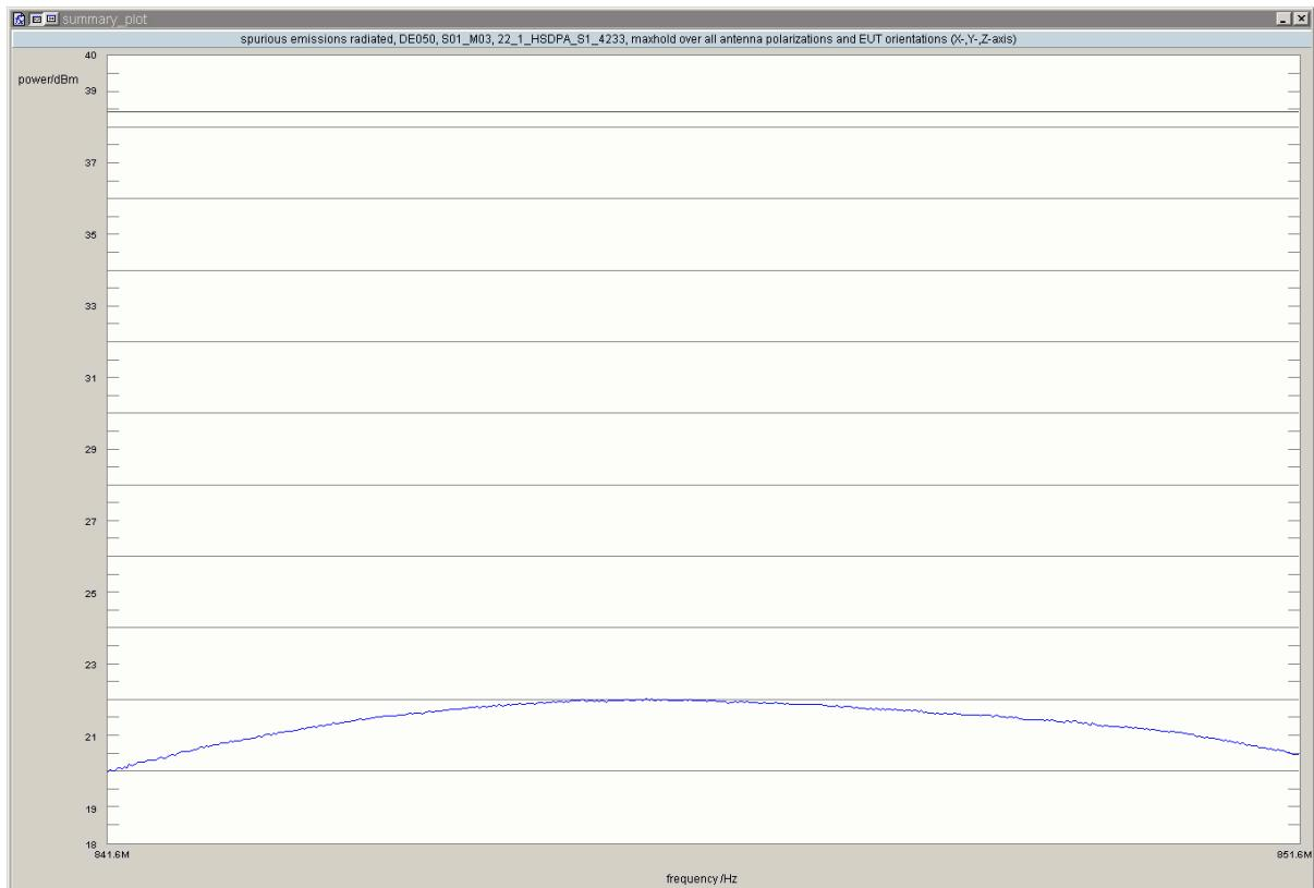
**Test: 22.1; Frequency Band = FDD5, Mode = HSDPA\_subtest\_2, Channel = 4132, Frequency = 826.4MHz, Method = conducted**
