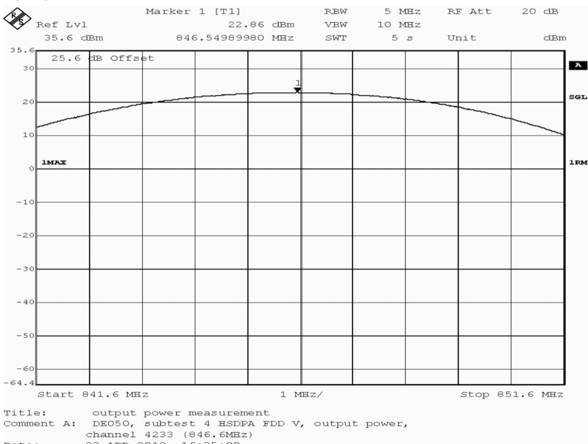
**Test: 22.1; Frequency Band = FDD5, Mode = HSDPA\_subtest\_4, Channel = 4233, Frequency = 846.6MHz, Method = radiated**
