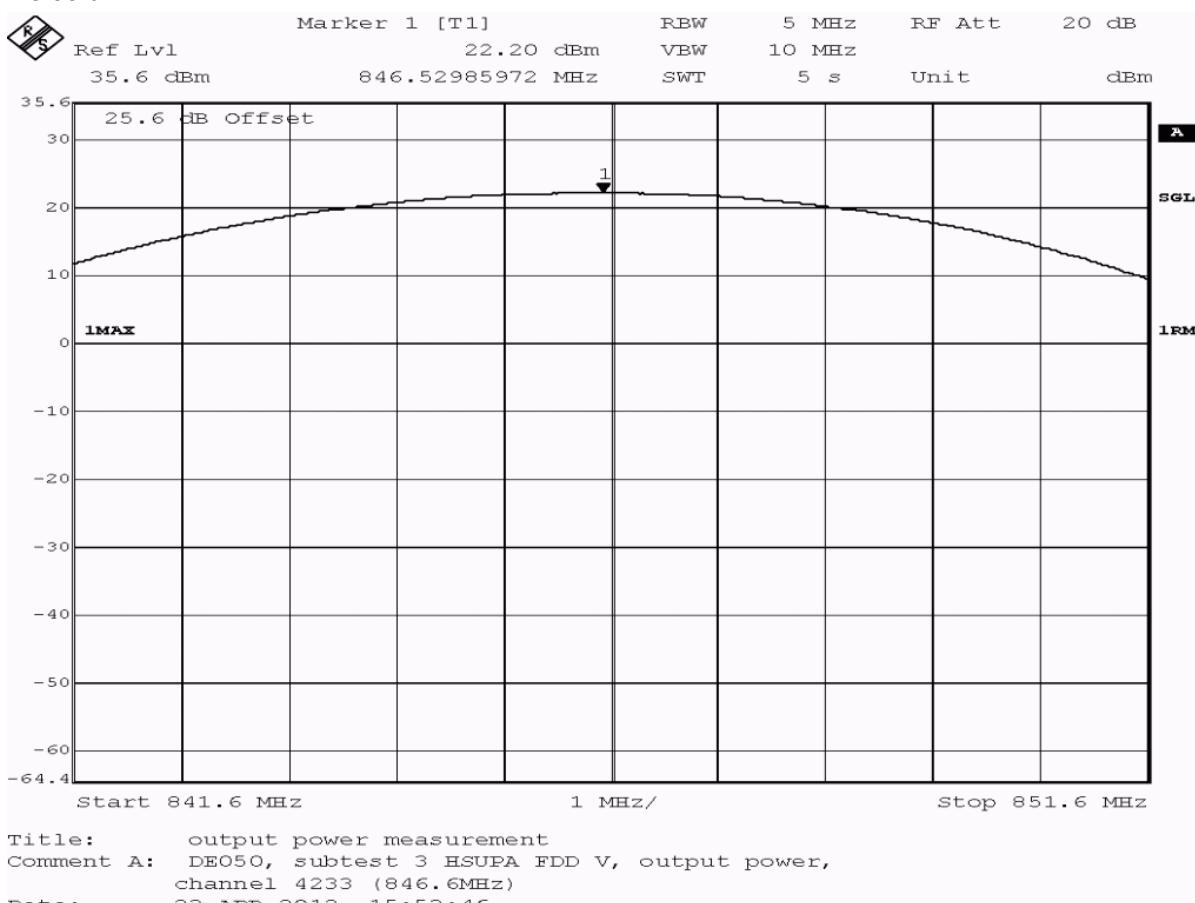
**Test: 22.1; Frequency Band = FDD5, Mode = HSUPA\_subtest\_3, Channel = 4233, Frequency = 846.6MHz, Method = radiated**
