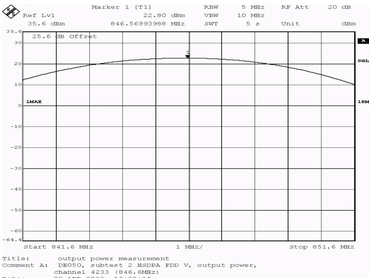
**Test: 22.1; Frequency Band = FDD5, Mode = HSDPA\_subtest\_2, Channel = 4233, Frequency = 846.6MHz, Method = radiated**
