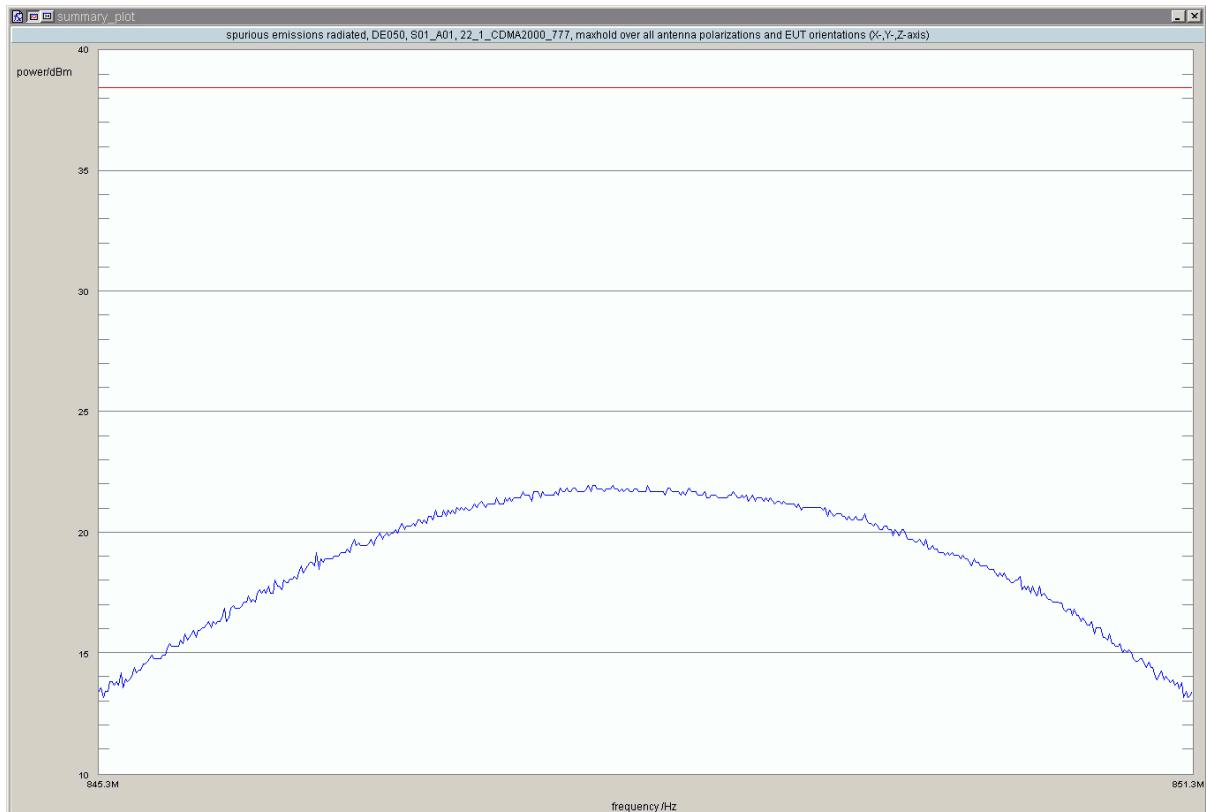
**Test: 22.1; Frequency Band = FDD5, Mode = HSDPA\_subtest\_1, Channel = 4132, Frequency = 826.4MHz, Method = conducted**
