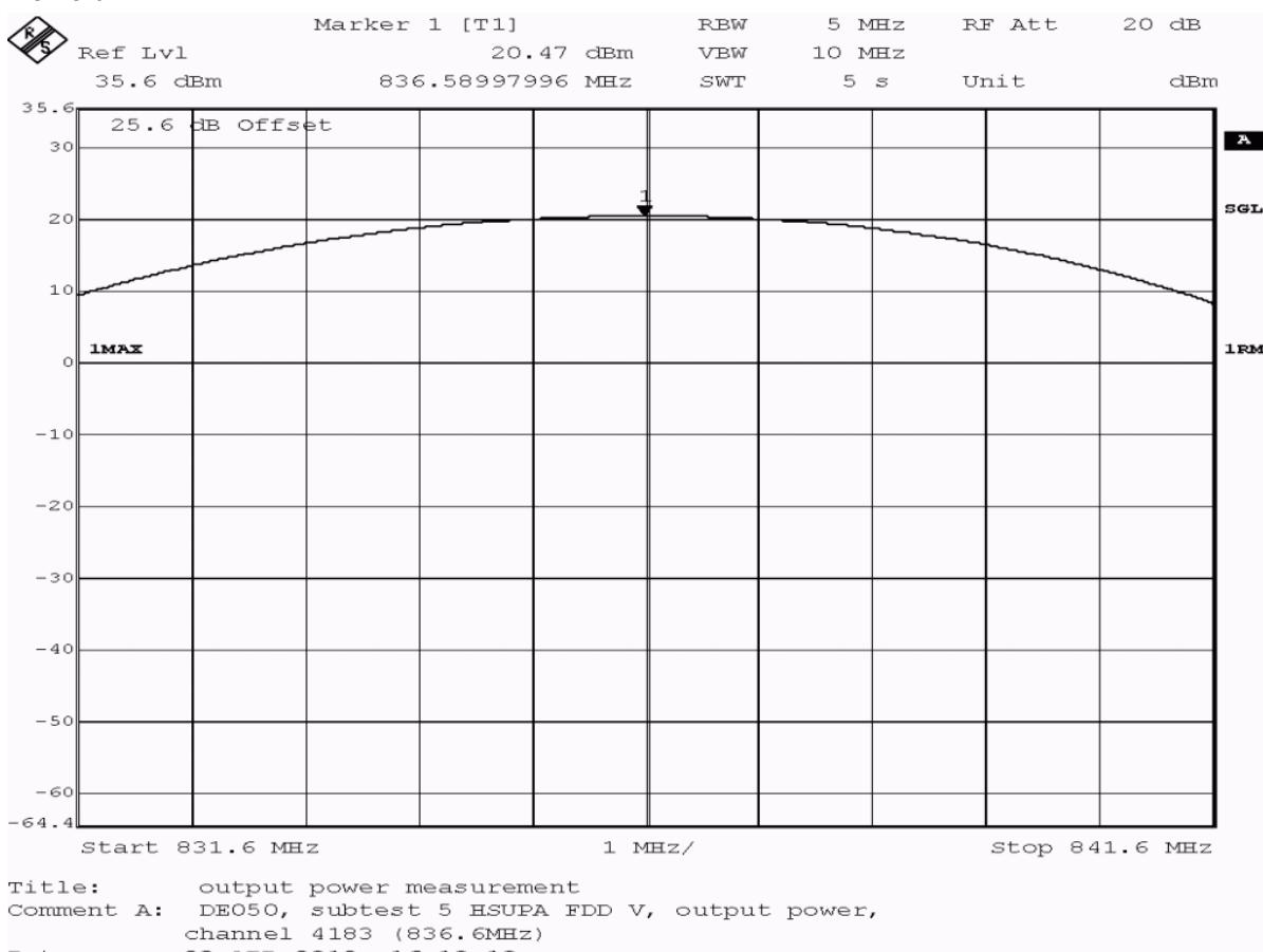
**Test: 22.1; Frequency Band = FDD5, Mode = HSUPA\_subtest\_5, Channel = 4183, Frequency = 836.6MHz, Method = radiated**
