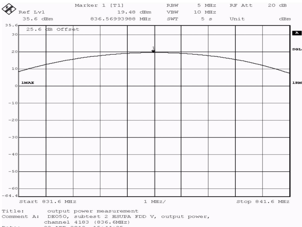
**Test: 22.1; Frequency Band = FDD5, Mode = HSUPA\_subtest\_2, Channel = 4183, Frequency = 836.6MHz, Method = radiated**
