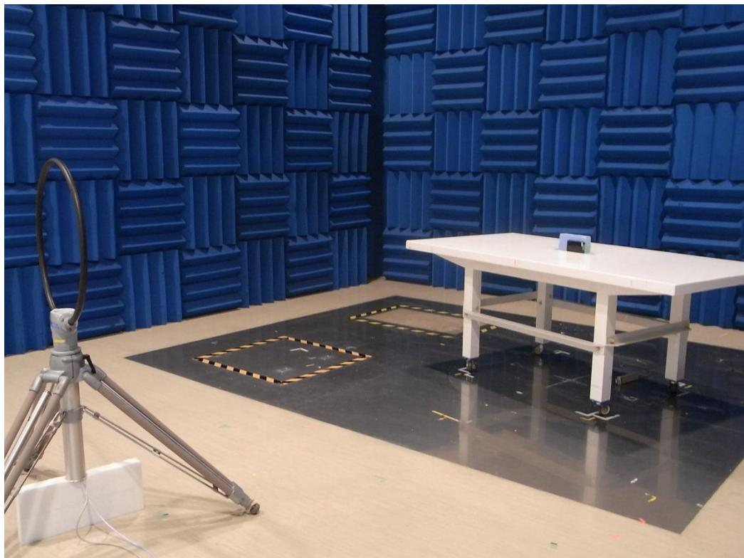
**Radiated Emission for 30MHz to 300MHz**
