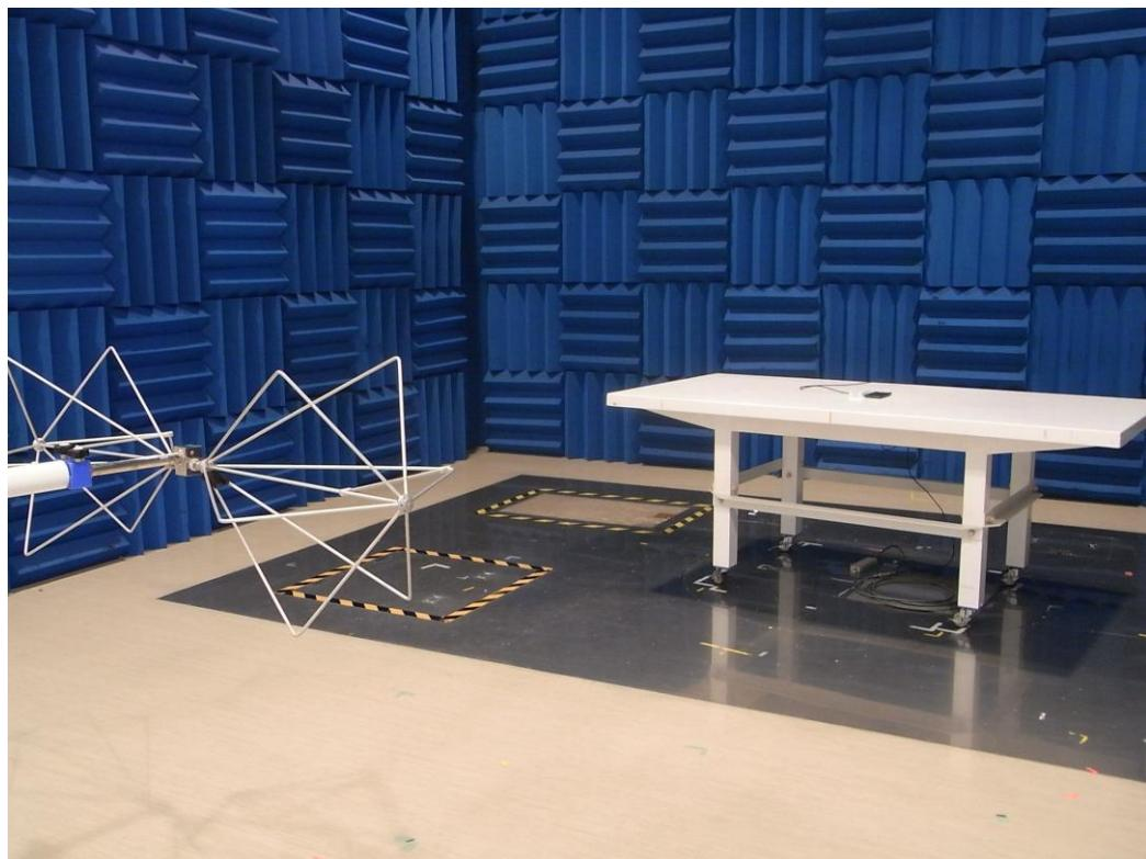
**Radiated Emission for 300MHz to 1GHz**
