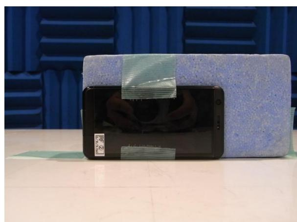
Note: X-axis generates the maximum emission at Bluetooth, 5GHz WLAN, GSM1900 and WCDMA Band II, LTE Band 17.
