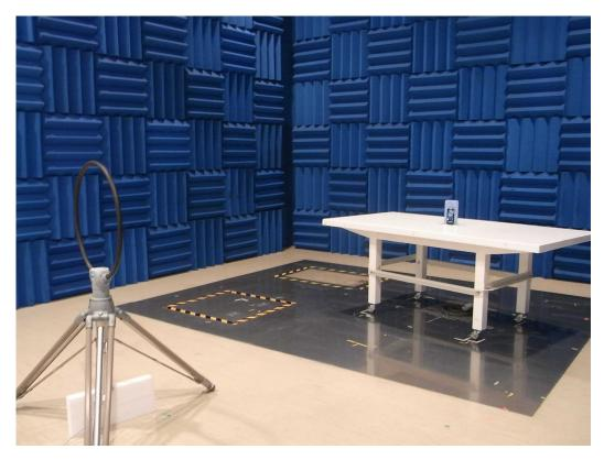
Radiated Emission for 30MHz to 300MHz
