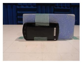
Note: X-axis generates the maximum emission at Bluetooth, GSM1900 and WCDMA Band II Y-axis generates the maximum emission at NFC.
