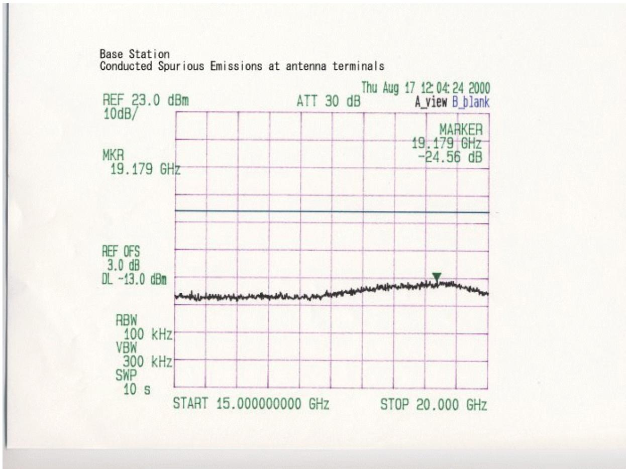
**6.5 TEST TYPE:** Spurious Emissions at Antenna Terminals at Block Edges +/- 1 MHz
