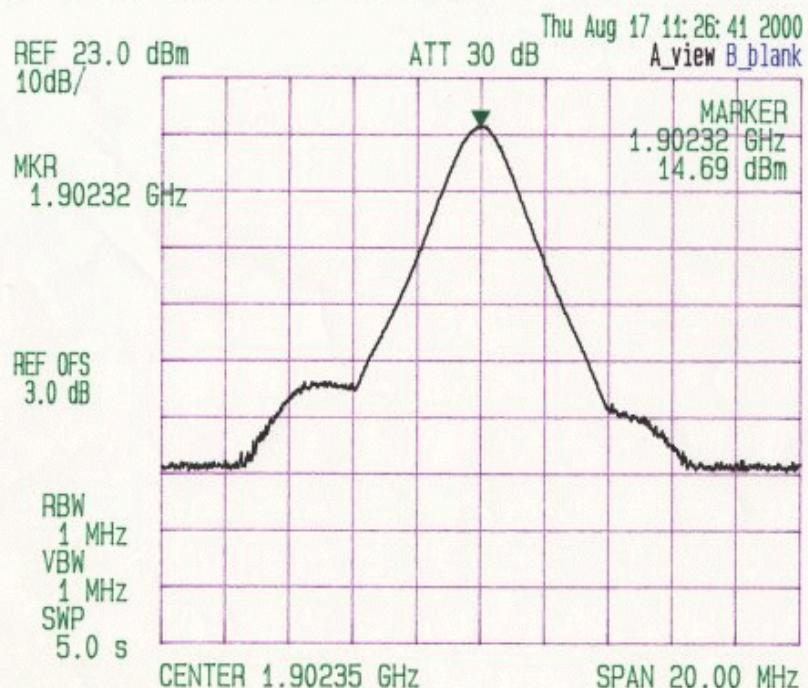
**6.4 TEST TYPE:** Spurious Emissions at Antenna Terminals**6.4.1 TECHNICAL SPECIFICATION:** 2.1051; 24.238(a)**6.4.2 TEST DATE(S):** 8/16/00**6.4.3 MEASUREMENT PROCEDURES:**
