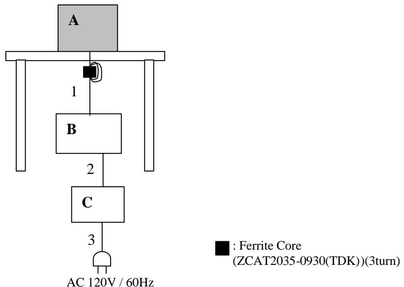
\* Cabling and setup were taken into consideration and test data was taken under worst case conditions.
