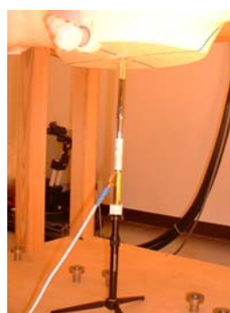
1800MHz System performance check setup
