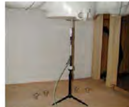
Figure 11.1 Dipole Verification Test Setup Diagram & Photo
