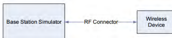
Figure 10.1 Power Measurement Setup
