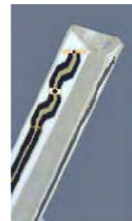
Figure 3.3 Probe Thick-Film Technique
