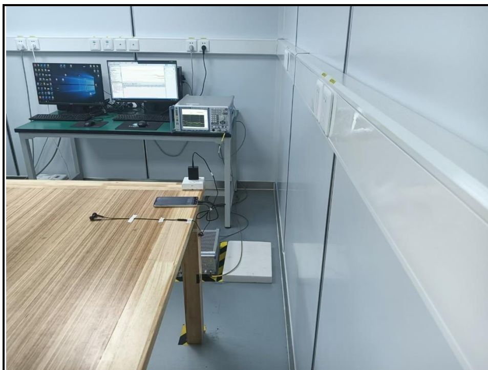
Fig. 4 Power line conducted emission setup photo
