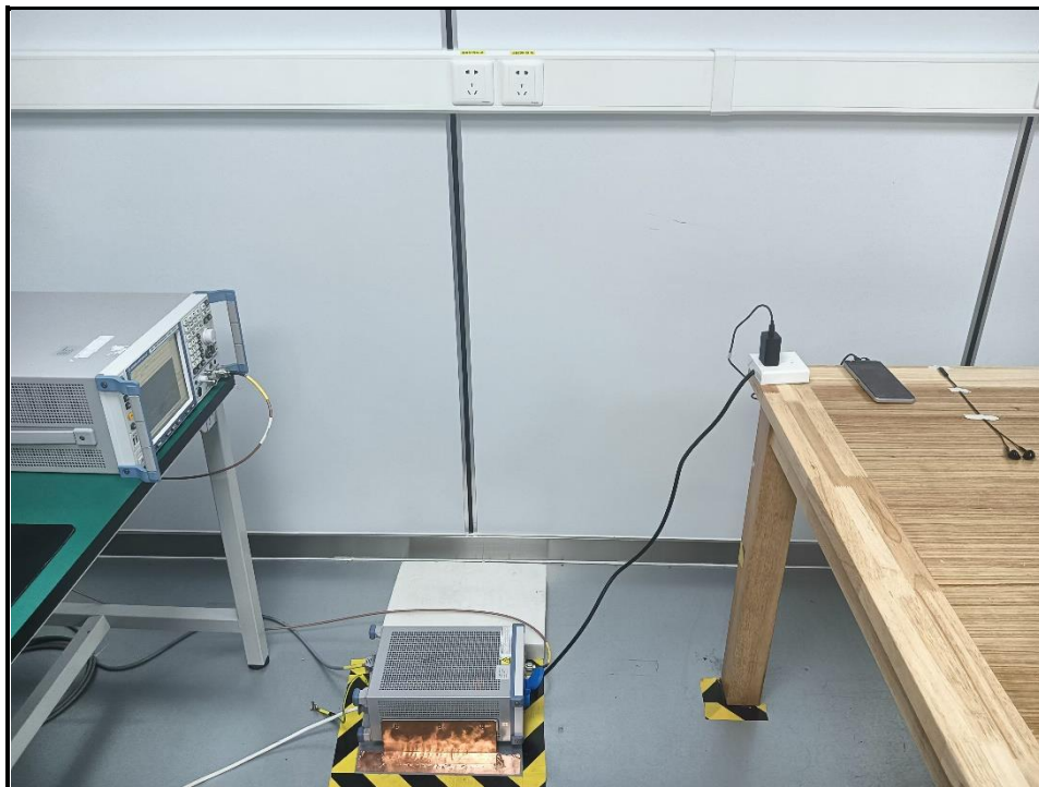
Fig. 3 Power line conducted emission setup photo
