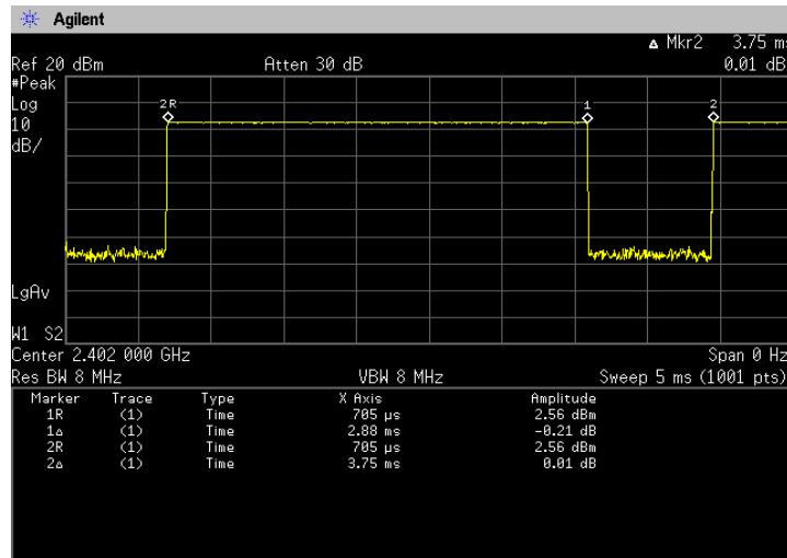
$$\text{Duty Cycle} = \text{Ton} / (\text{Ton} + \text{Toff}) = 2880[\mu\text{s}] / (2880[\mu\text{s}] + 870[\mu\text{s}]) = 76.8[\%]$$
