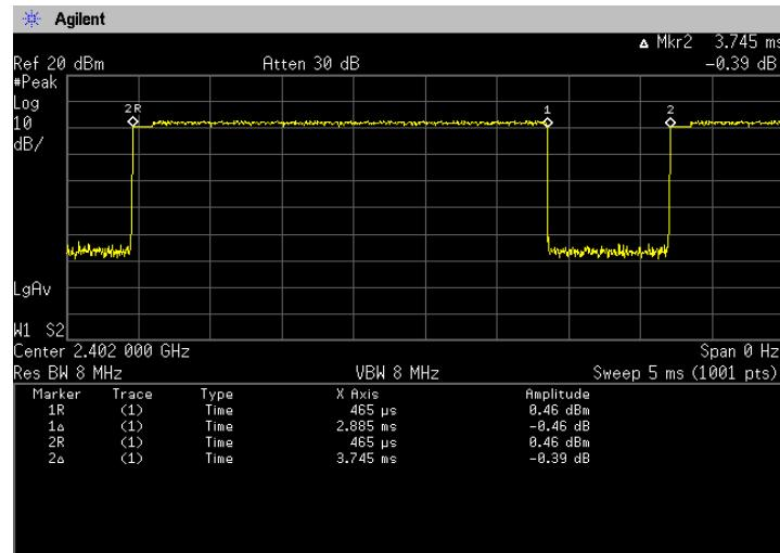
$$\text{Duty Cycle} = \text{Ton} / (\text{Ton} + \text{Toff}) = 2885[\mu\text{s}] / (2885[\mu\text{s}] + 860[\mu\text{s}]) = 77.04[\%]$$
