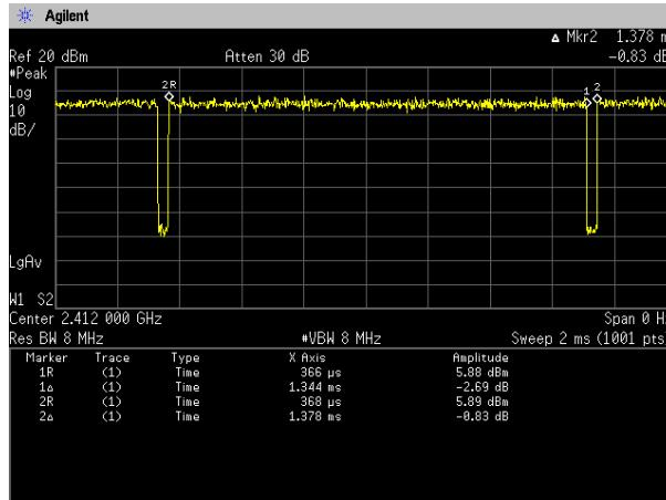
$$\text{Duty Cycle} = \text{Ton} / (\text{Ton} + \text{Toff}) = 1344[\mu\text{s}] / (1344[\mu\text{s}] + 34[\mu\text{s}]) = 97.53\%]$$
