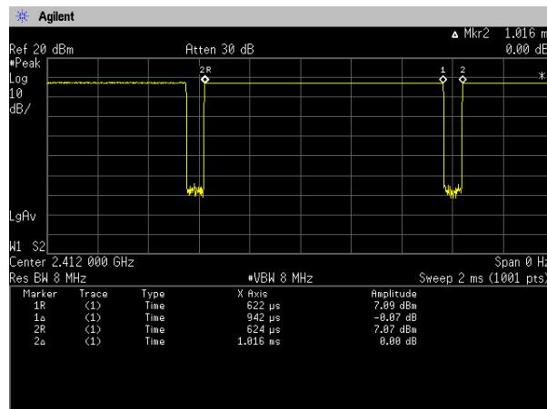
$$\text{Duty Cycle} = \text{Ton} / (\text{Ton} + \text{Toff}) = 942[\mu\text{s}] / (942[\mu\text{s}] + 74[\mu\text{s}]) = 92.72\%]$$
