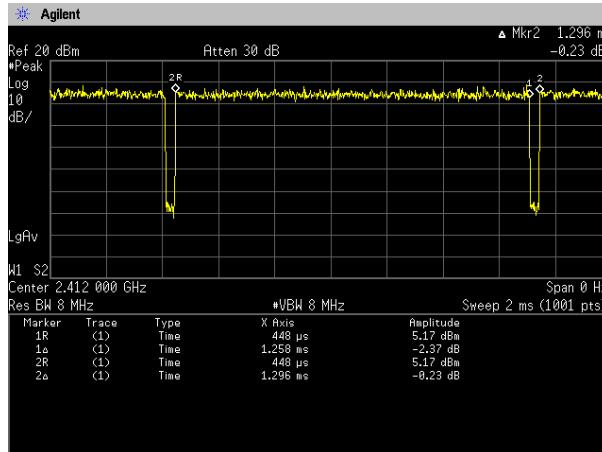
$$\text{Duty Cycle} = \text{Ton} / (\text{Ton} + \text{Toff}) = 1258[\mu\text{s}] / (1258[\mu\text{s}] + 38[\mu\text{s}]) = 97.07\%]$$
