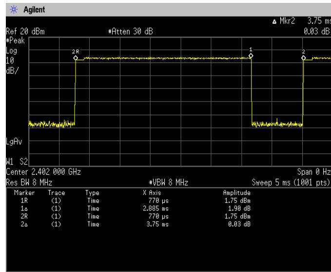
$$\text{Duty Cycle} = T_{on} / (T_{on} + T_{off}) = 2885[\mu\text{s}] / (2885[\mu\text{s}] + 865[\mu\text{s}]) = 76.93\%[ ]$$
