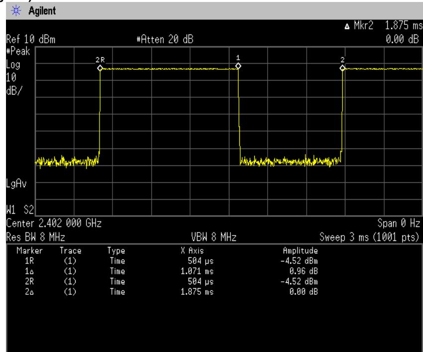
$$\text{Duty Cycle} = \text{Ton} / (\text{Ton} + \text{Toff}) = 1071[\mu\text{s}] / (1071[\mu\text{s}] + 804[\mu\text{s}]) = 57.12[\%]$$
