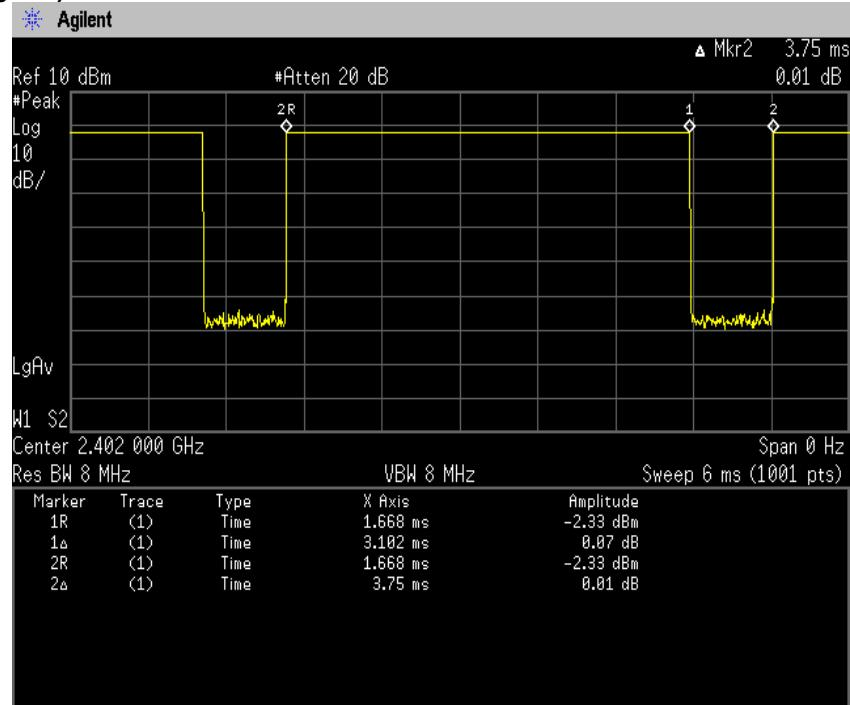
$$\text{Duty Cycle} = \text{Ton} / (\text{Ton} + \text{Toff}) = 3102[\mu\text{s}] / (3102[\mu\text{s}] + 648[\mu\text{s}]) = 82.72[\%]$$
