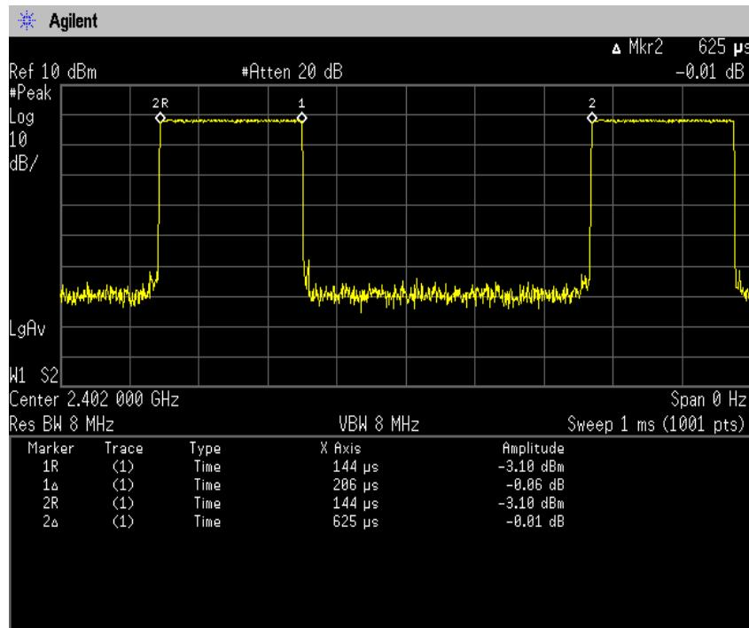
$$\text{Duty Cycle} = \text{Ton} / (\text{Ton} + \text{Toff}) = 206[\mu\text{s}] / (206[\mu\text{s}] + 419[\mu\text{s}]) = 32.96[\%]$$
