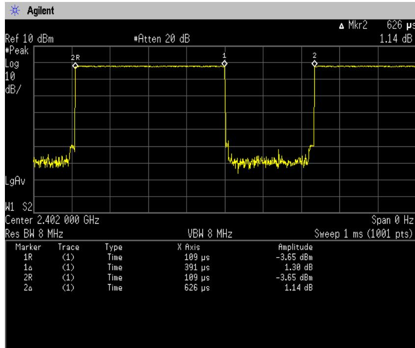
$$\text{Duty Cycle} = \text{Ton} / (\text{Ton} + \text{Toff}) = 391[\mu\text{s}] / (391[\mu\text{s}] + 235[\mu\text{s}]) = 62.46[\%]$$
