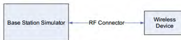
Figure 9.1 Power Measurement Setup
