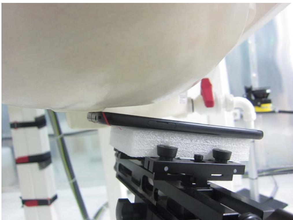
**■ Test Setup Photo (Head SAR Test Photo)**
