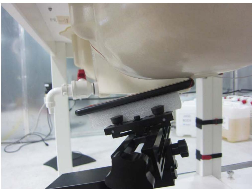
**■ Test Setup Photo (Body SAR Test Photo)**
