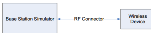
Figure 10.1 Power Measurement Setup
