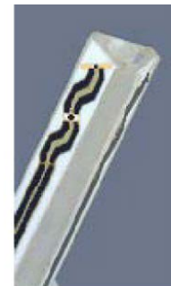
Figure 3.3 Probe Thick-Film Technique
