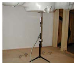
Figure 11.1 Dipole Verification Test Setup Diagram & Photo
