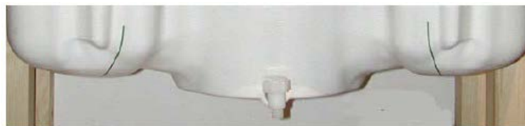
Figure 3.7 Sam Twin Phantom shell
