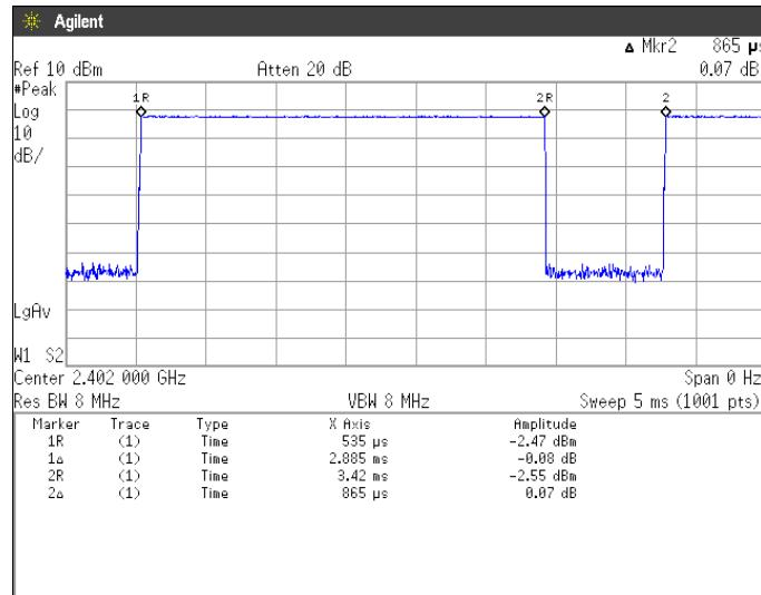
$$\text{Duty Cycle} = \text{Ton} / (\text{Ton} + \text{Toff}) = 2885[\mu\text{s}] / (2885[\mu\text{s}] + 865[\mu\text{s}]) = 76.93[\%]$$
