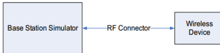
Figure 10.2 Power Measurement Setup
