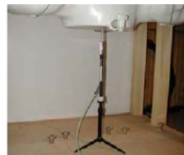
Figure 11.1 Dipole Verification Test Setup Diagram & Photo
