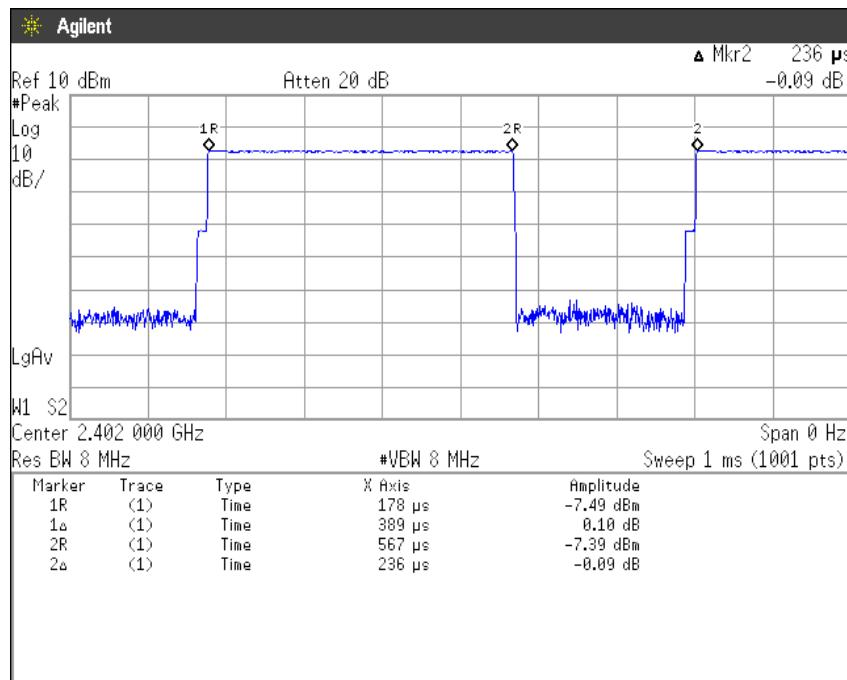
$$\text{Duty Cycle} = \text{Ton} / (\text{Ton} + \text{Toff}) = 389[\mu\text{s}] / (389[\mu\text{s}] + 236[\mu\text{s}]) = 62.24[\%]$$
