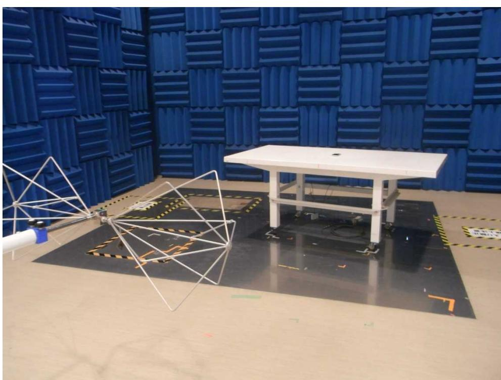
**Radiated Emission for 300MHz to 1GHz**
