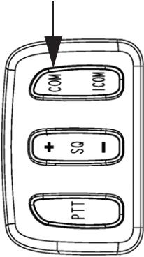
Push COM or ICOM on the left control or (+) or (-) on the console panel to change channels.
