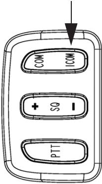
When the intercom system is active, ICOM will display on the console screen.
