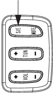
Press S/E on the left control to exit the screen and return to the main display.
