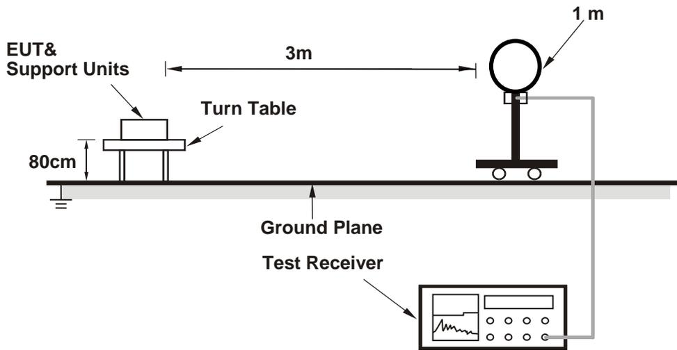
**For Radiated emission 30MHz to 1GHz**
