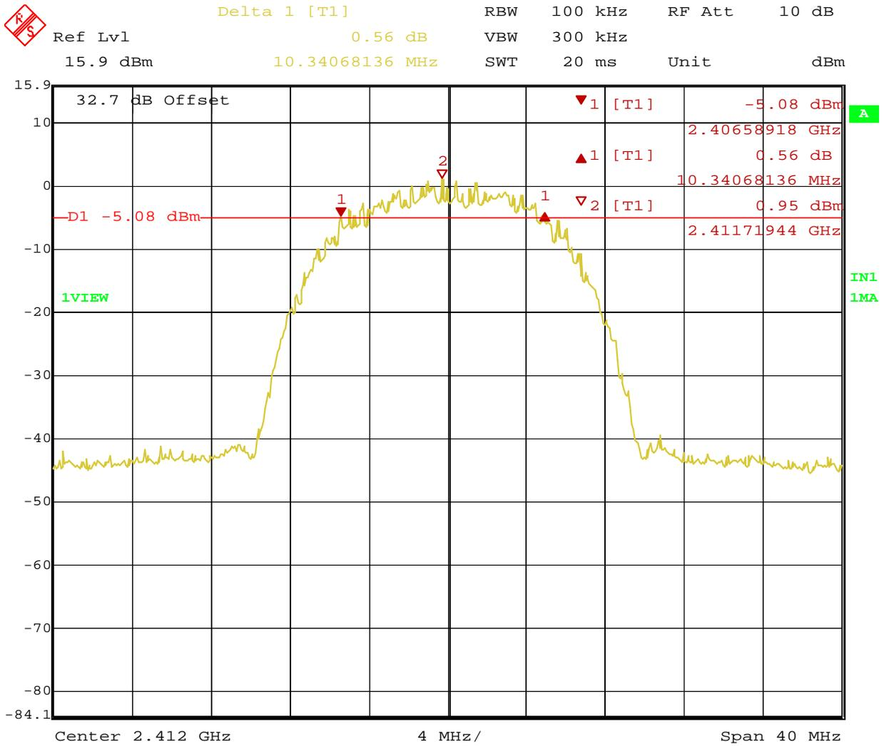
**Figure 8:** 6dB Bandwidth at 11Mbit/s – Operating Channel 2412 MHz (Vertical)
