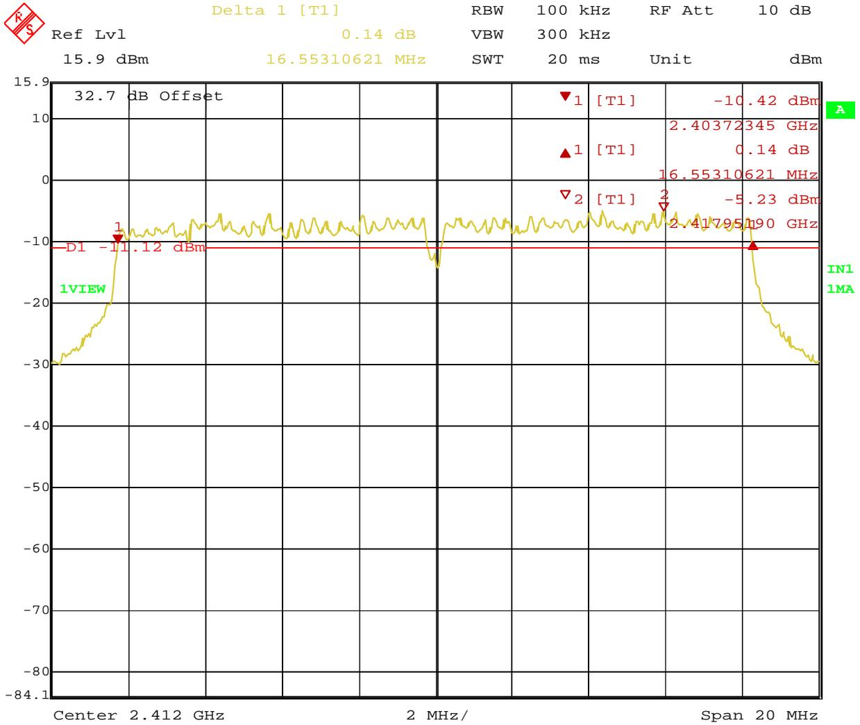
**Figure 14:** 6dB Bandwidth at 54Mbit/s – Operating Channel 2412 MHz (Vertical)
