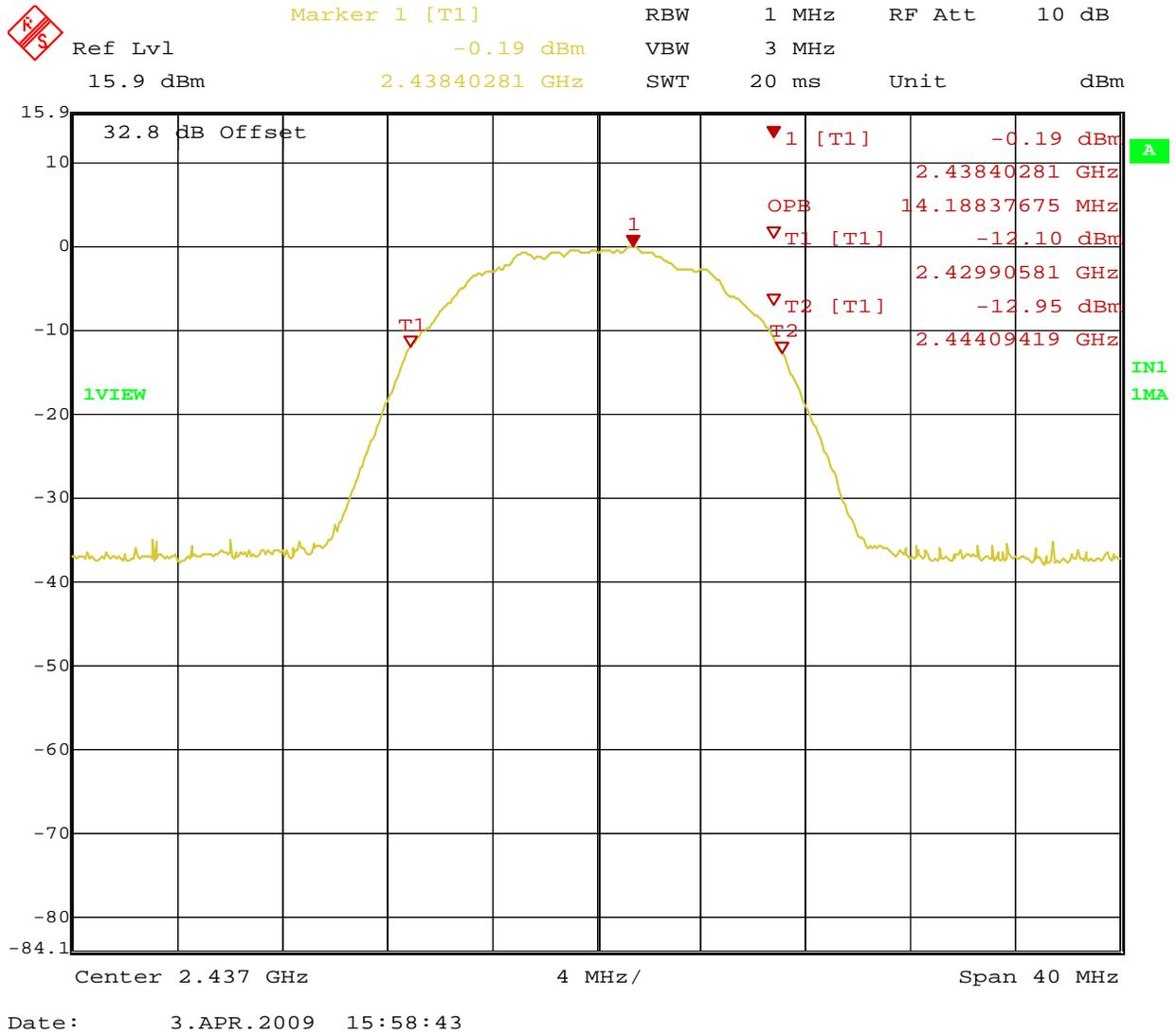
**Figure 21:** 99% Bandwidth at 11Mbit/s – Operating Channel 2437 MHz (Horizontal)
