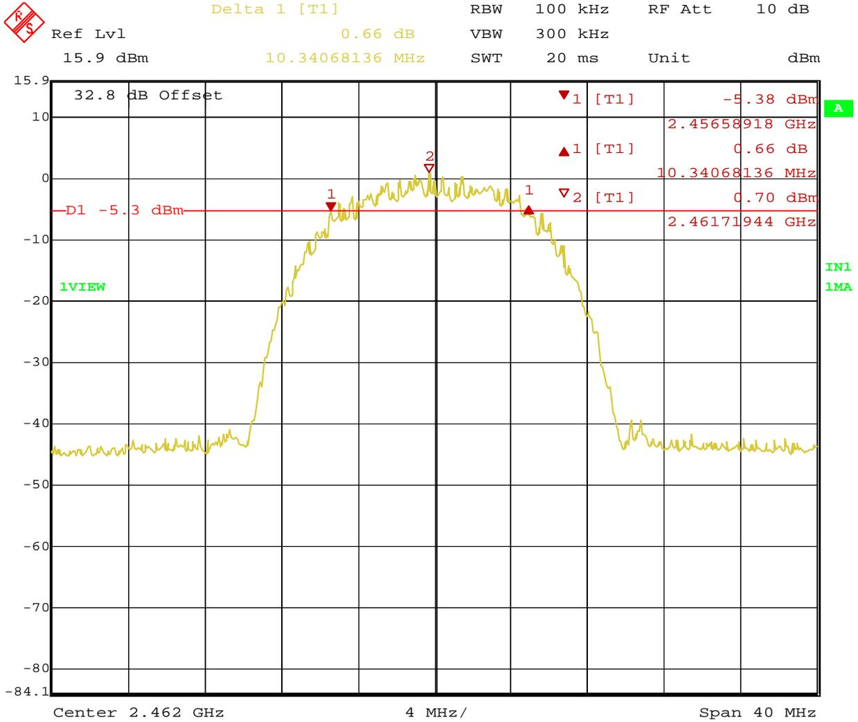
**Figure 12:** 6dB Bandwidth at 11Mbit/s – Operating Channel 2462 MHz (Vertical)
