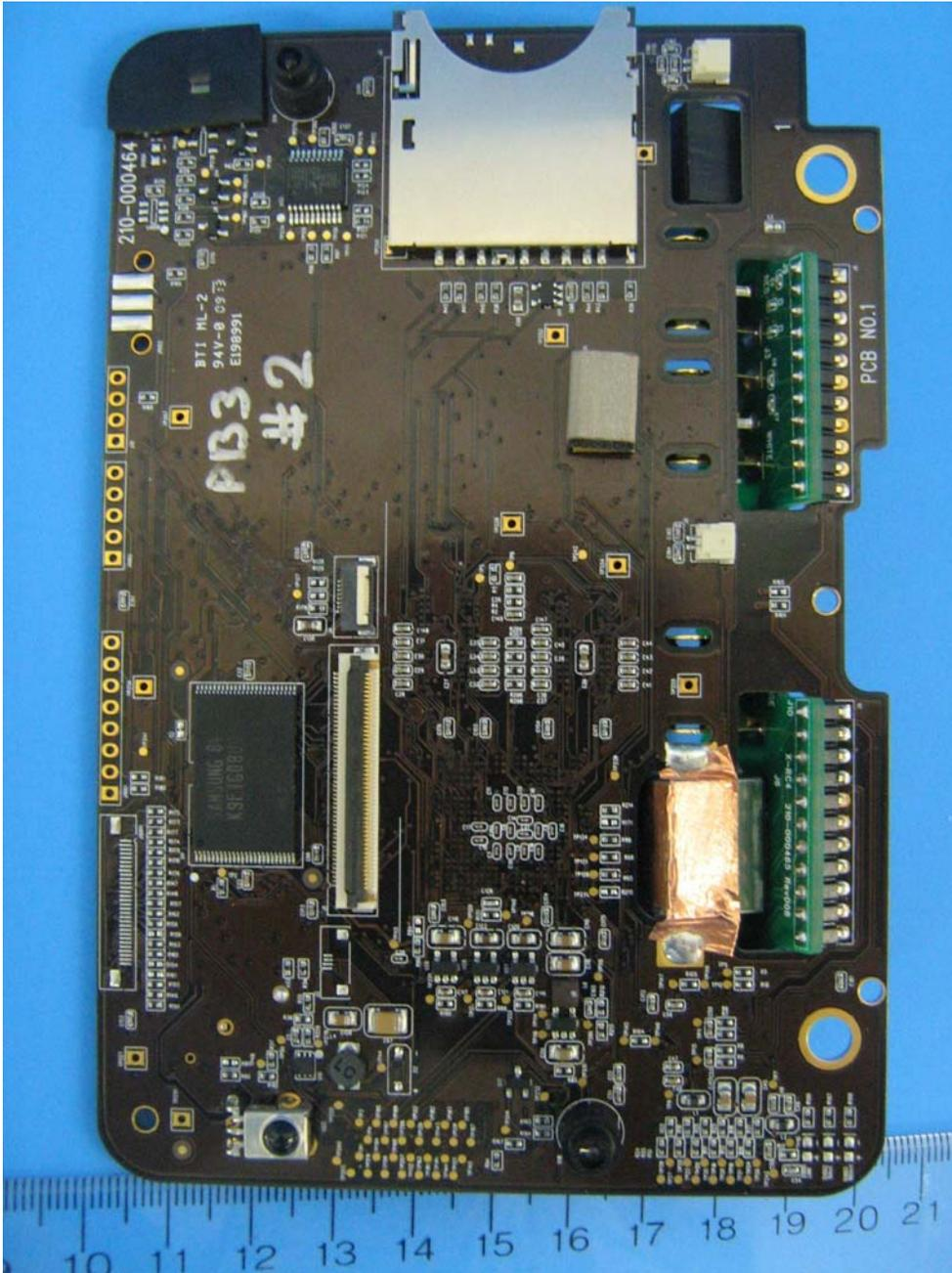
**Figure 12:** Internal Photo of X-RC4 - PCB Board (Front Side)
