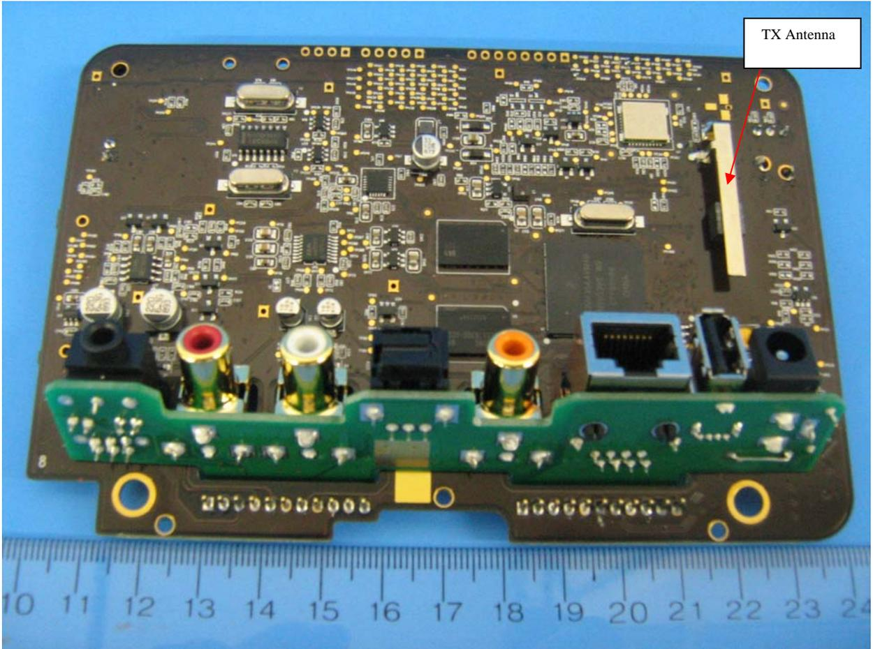
**Figure 13:** Internal Photo of X-RC4 - PCB Board (Rear Side)
