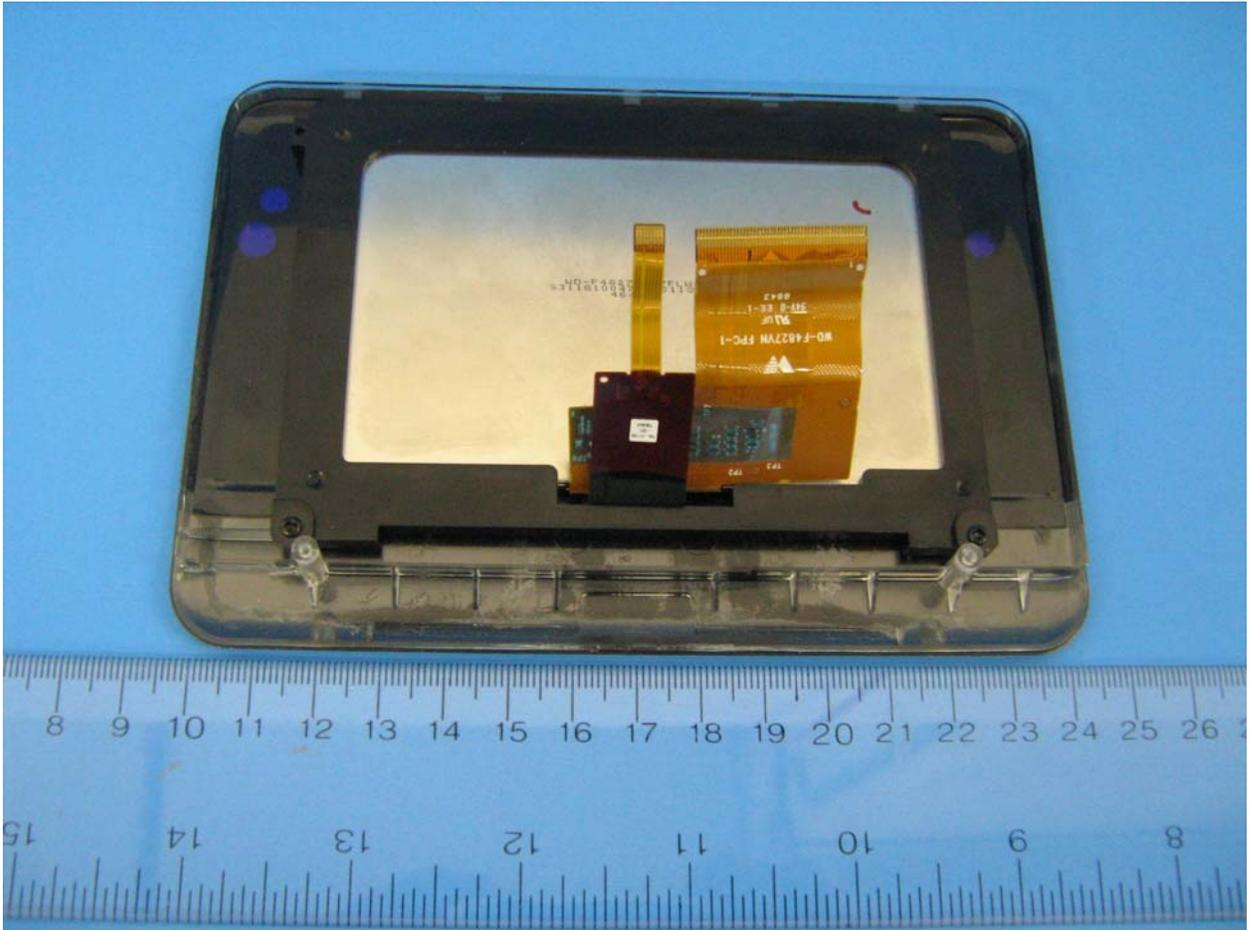
**Figure 11:** Internal Photo of X-RC4 – LCD
