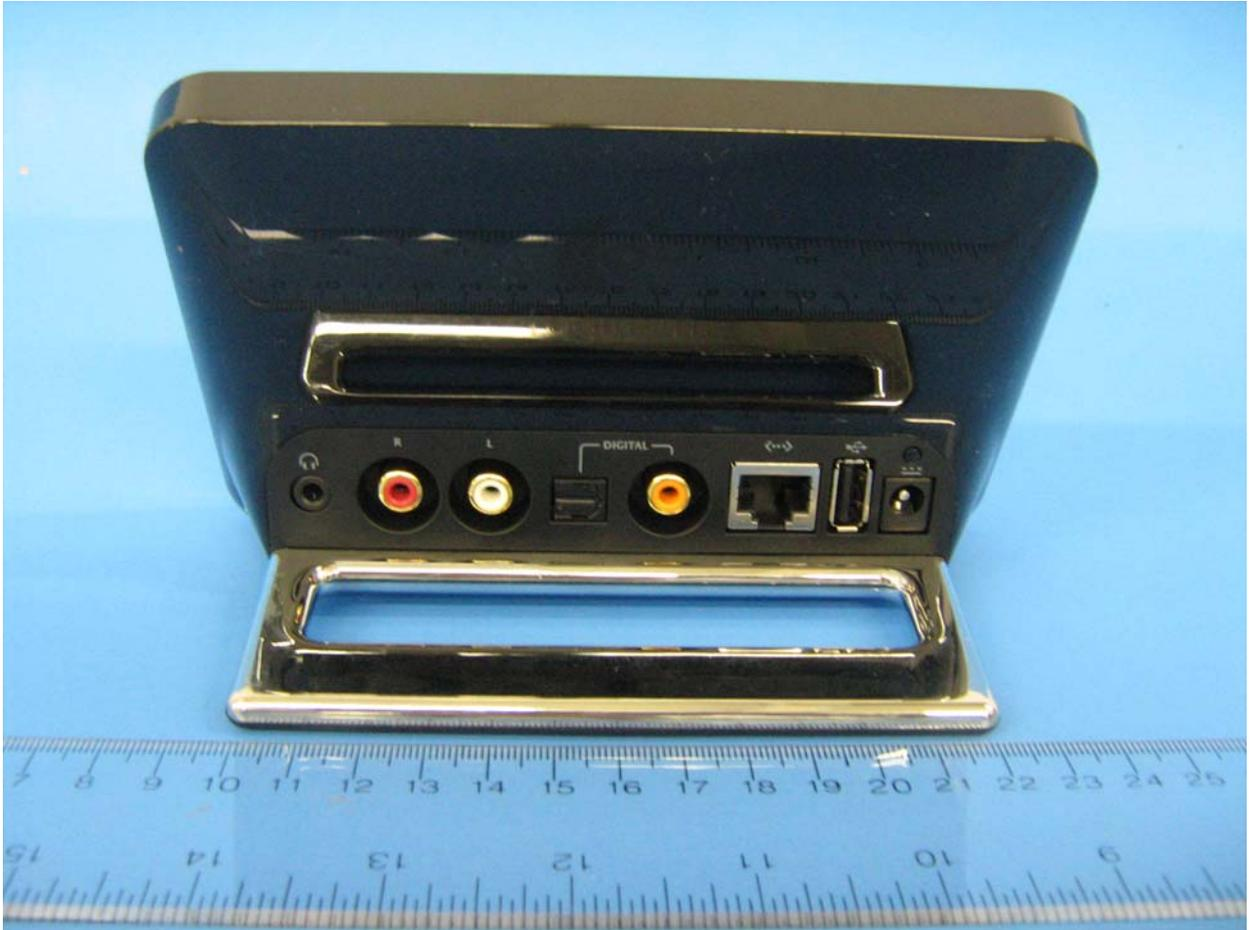
**Figure 9:** External Photo of X-RC4 – Rear View
