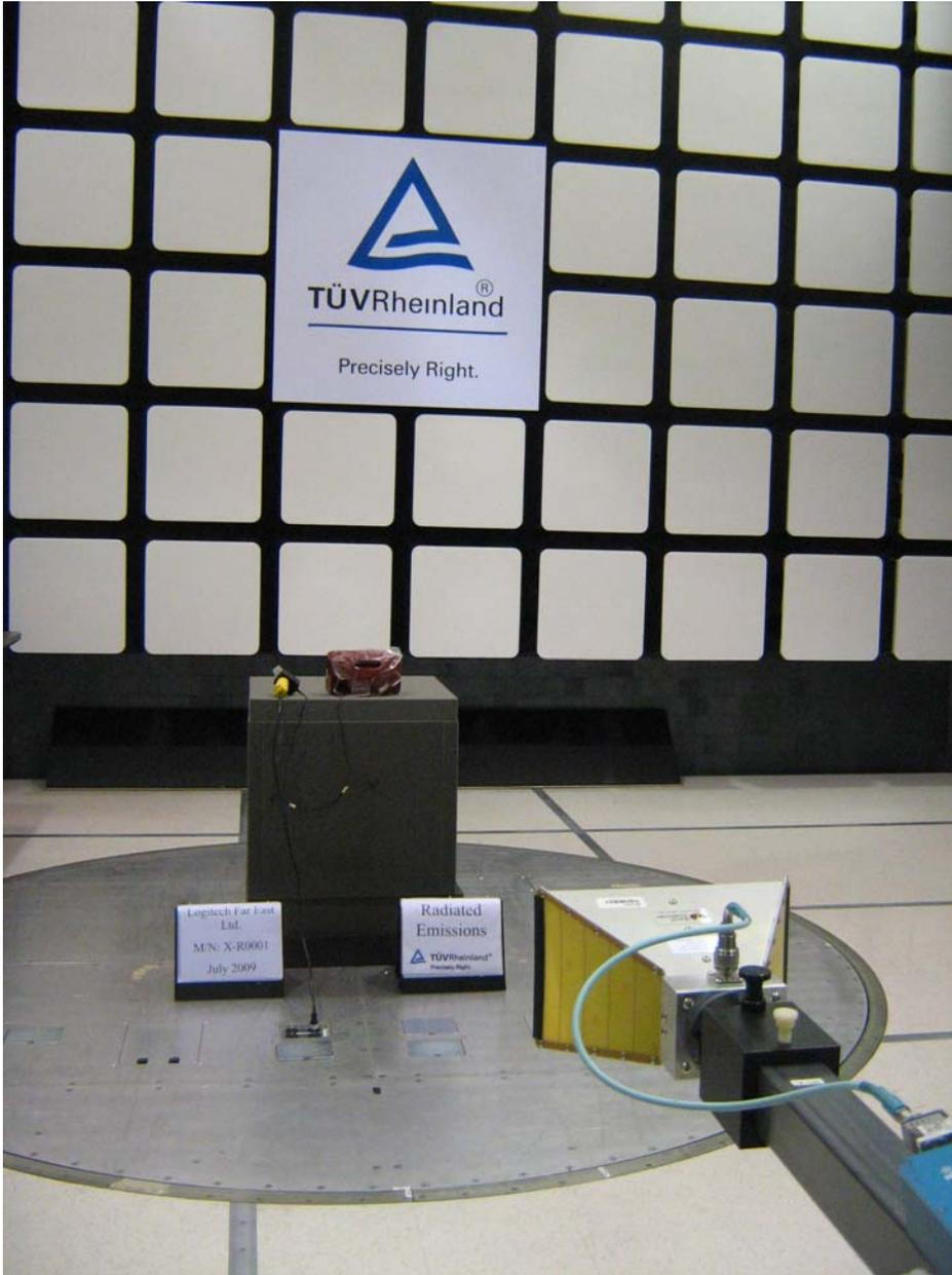
**Figure 4:** Photo of Test Setup for X-R0001, 1GHz to 18GHz (Rear View)
