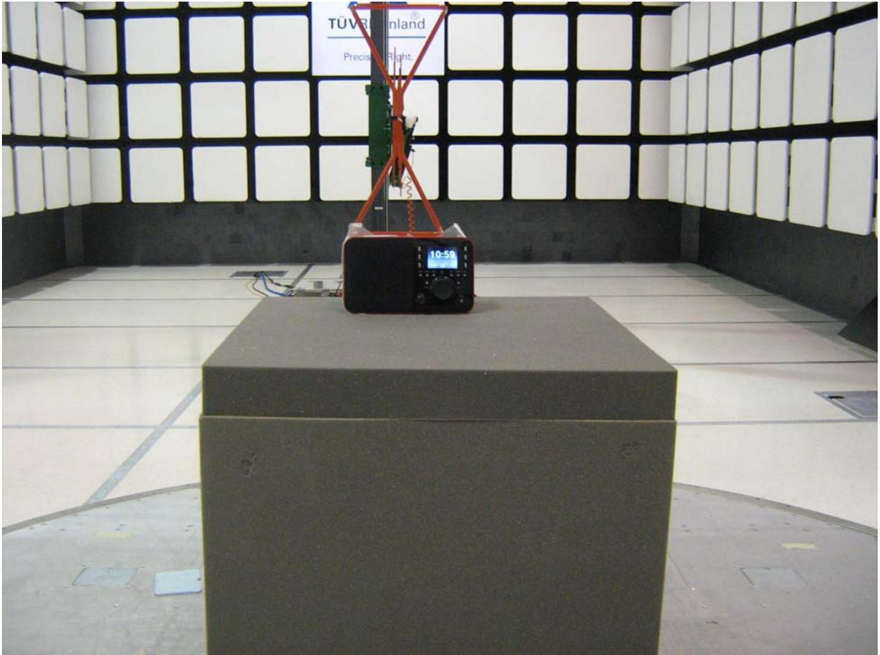
**Figure 1:** Photo of Test Setup for X-R0001, 30 MHz to 1000MHz (Front View)
