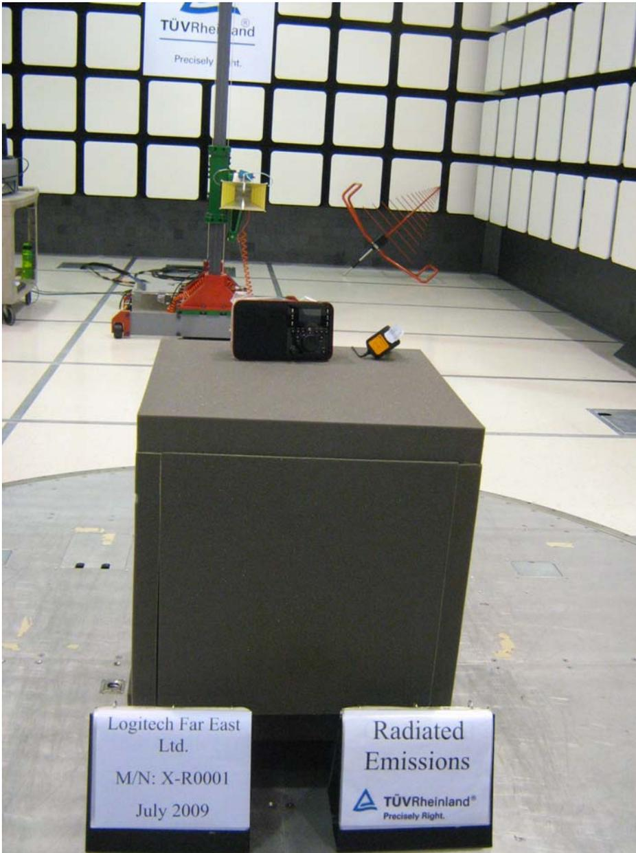
**Figure 3:** Photo of Test Setup for X-R0001, 1GHz to 18GHz (Front View)
