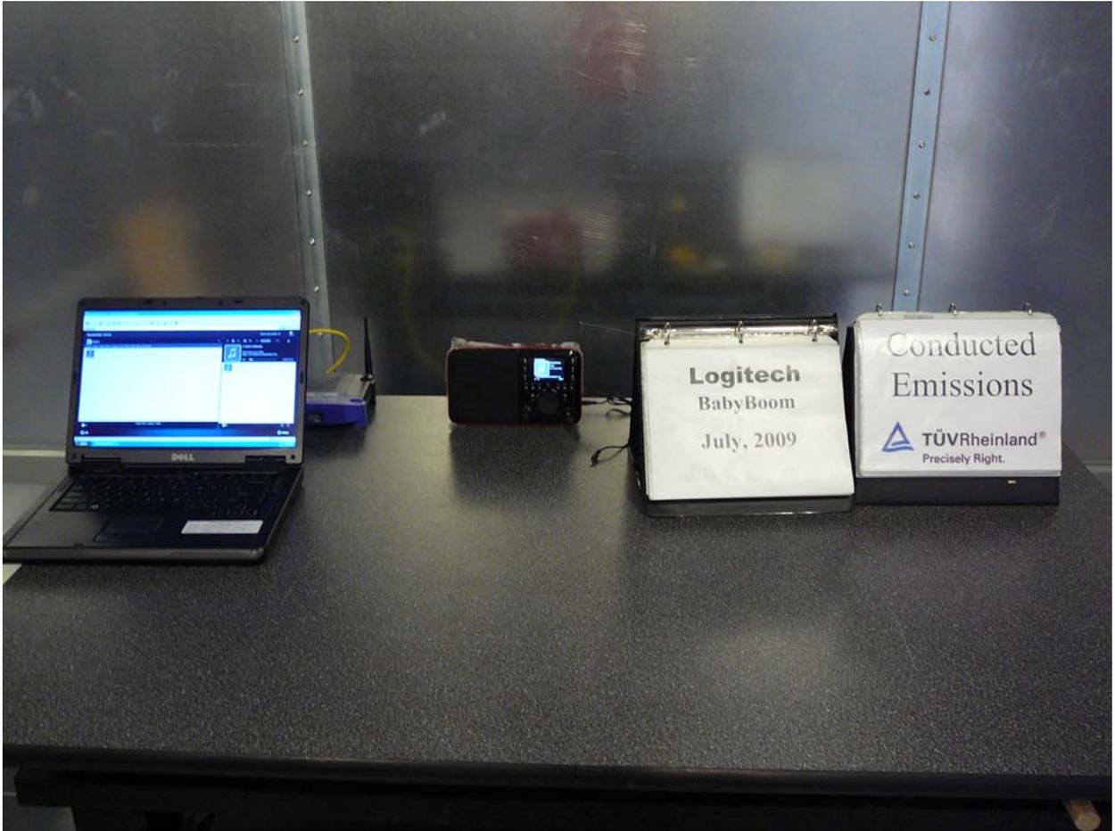
**Figure 7:** Photo of Test Setup for X-R0001, AC Conducted Emission (Front View)
