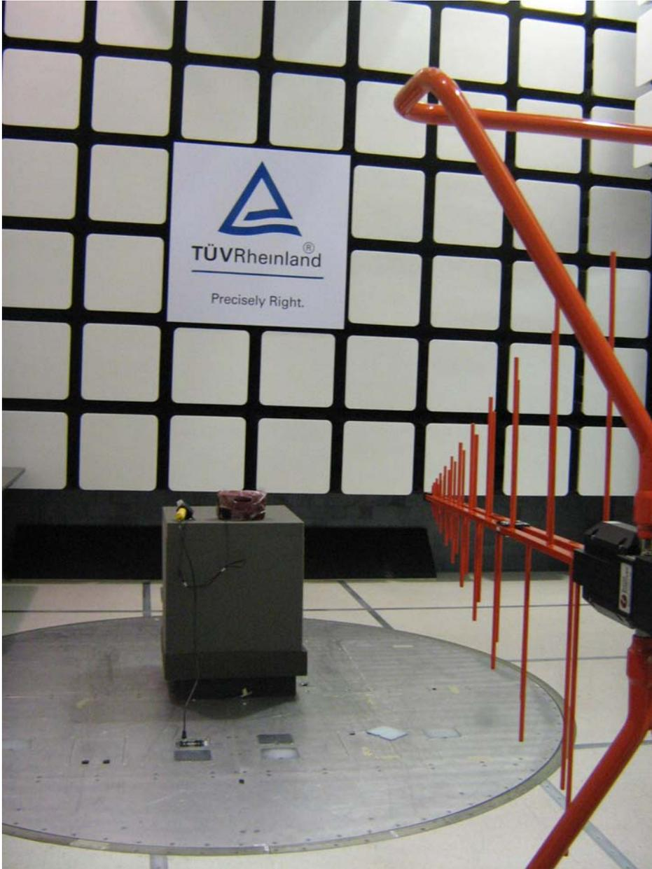
**Figure 2:** Photo of Test Setup for X-R0001, 30 to 1000 MHz (Rear View)
