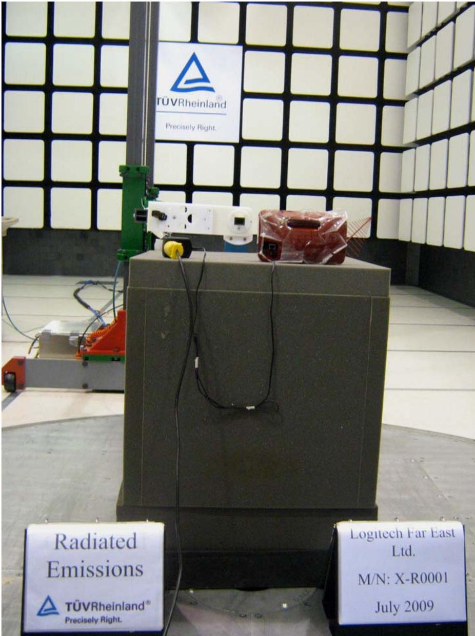
**Figure 6:** Photo of Test Setup for X-R0001, 18 GHz to 26GHz (Rear View)
