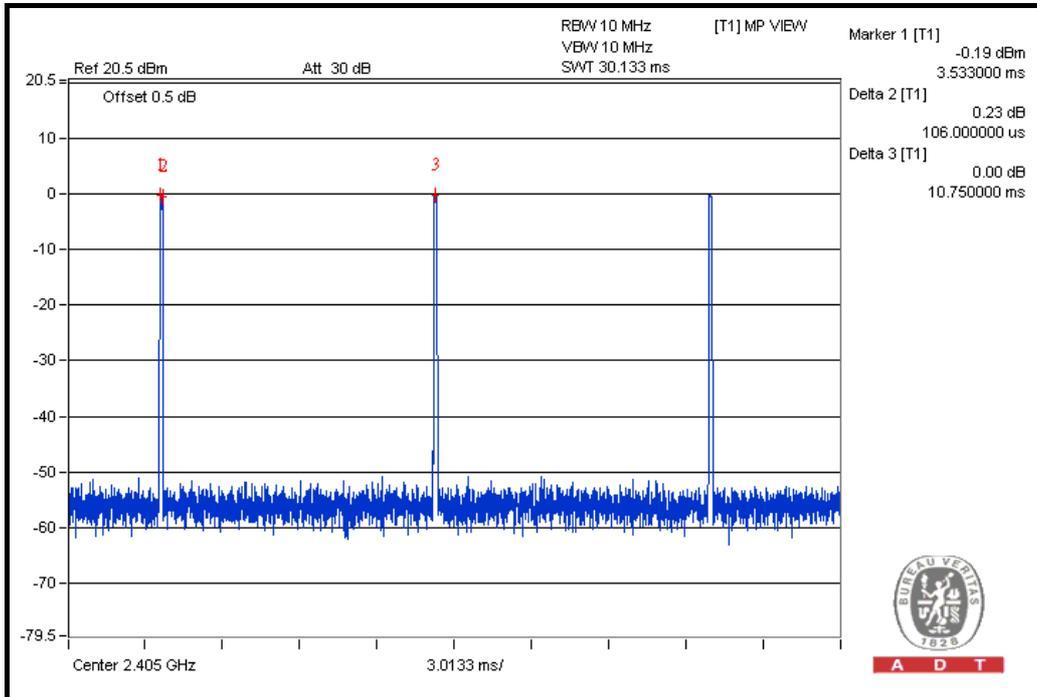
$$20 \log (\text{Duty cycle}) = 20 \log (0.106 \text{ ms} / 10.75 \text{ ms}) = -40.1 \text{ dB}$$
