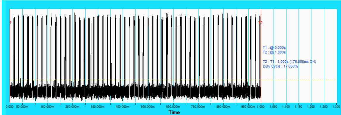
**NOTE:** T1 denotes the start of duty cycle period is 0<sup>th</sup> second. T2 denotes the end of duty cycle period is 1<sup>th</sup> second. T2 – T1= 1 seconds. Duty Cycle = 17.650%
