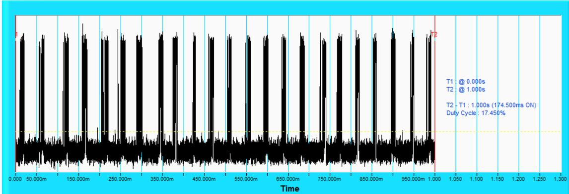
**NOTE:** T1 denotes the start of duty cycle period is 0<sup>th</sup> second. T2 denotes the end of duty cycle period is 1<sup>th</sup> second. T2 – T1= 1 seconds. Duty Cycle = 17.450%
