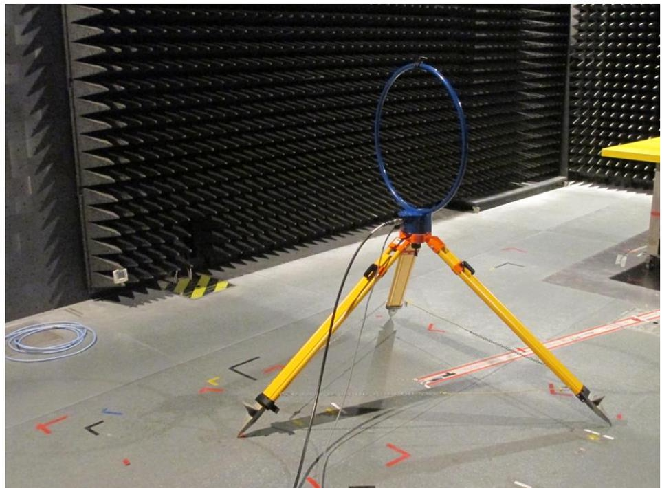
For radiated emissions 30MHz~1GHz
