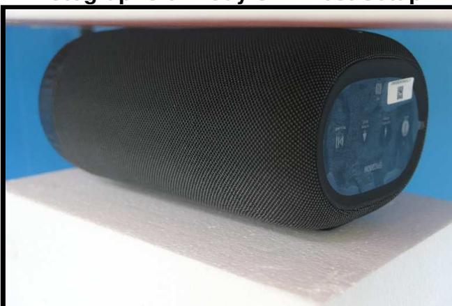
Front Face of EUT Tested at 0 mm
